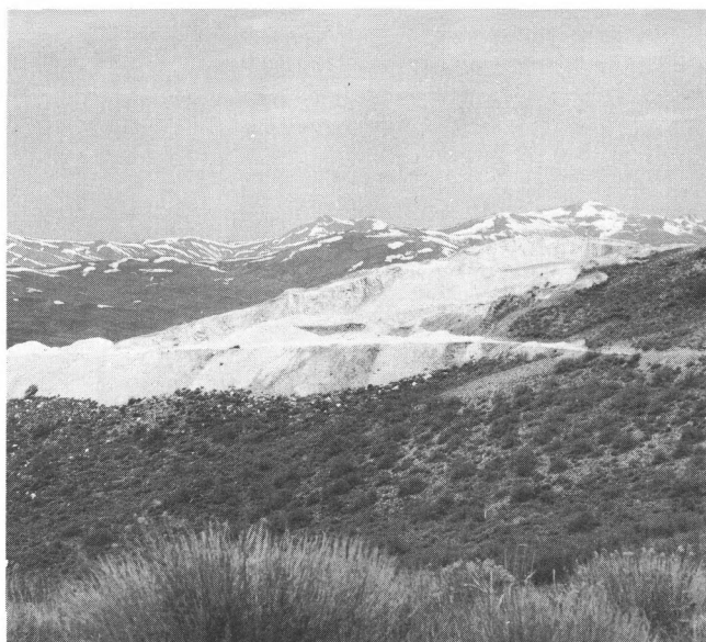
P 38. Quarry in the Eureka Quartzite? in the Dove Creek Mountains. The rock is crushed and sized for use as white garden stone.
