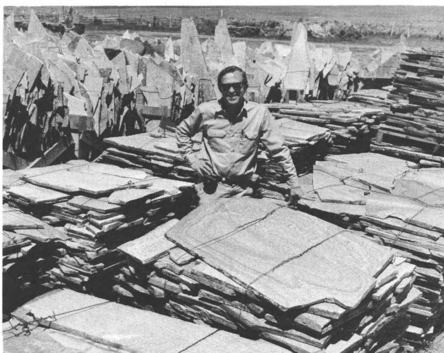
P 33. Pallets of flagstone, dimension stone quarried in the Vipont Mountains. The source rock is the Quartzite of Clarks Basin.
