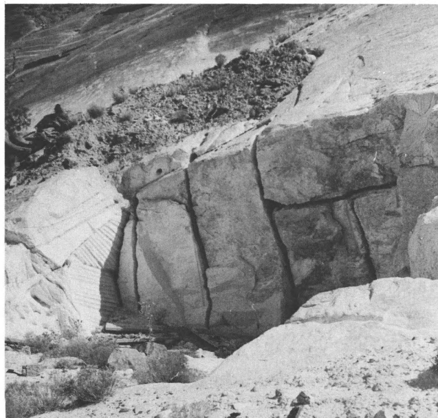
P 35. Pure white marble quarried by closely spaced drilling. Only small tonnages of this rock have been produced in the New-foundland Mountains.
