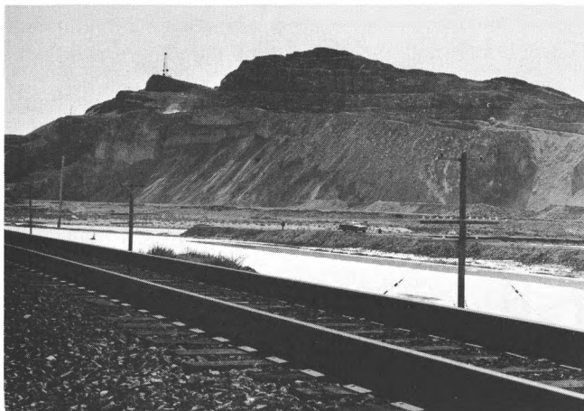
P 34. Lakeside No. 2 quarry of the Southern Pacific Railroad. This quarry is used as riprap and railroad ballast.
