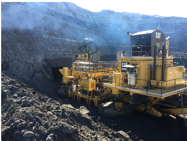
Figure 11. Highwall mining machine currently in use at the Coal Hollow open pit mine in southern Utah.
