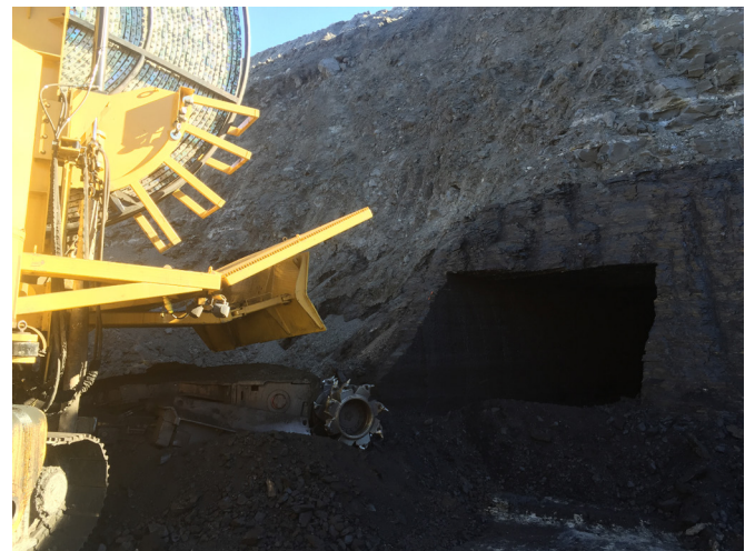
Figure 11. Highwall mining machine currently in use at the Coal Hollow open pit mine in southern Utah.
