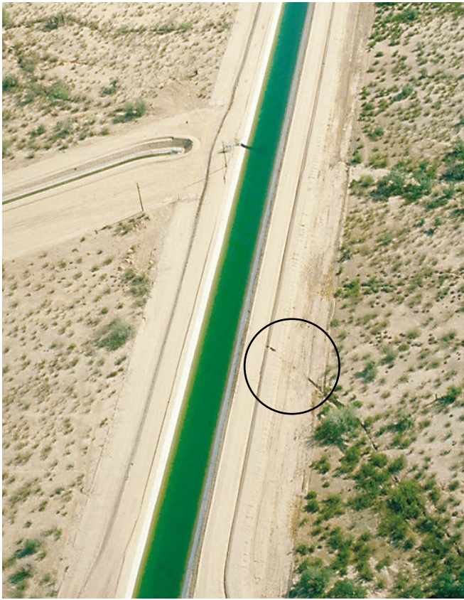
Figure 37. Earth fissure intersecting an irrigation canal embankment near Phoenix, Arizona. Photo credit U.S. Bureau of Reclamation (after Carpenter, 1999).
