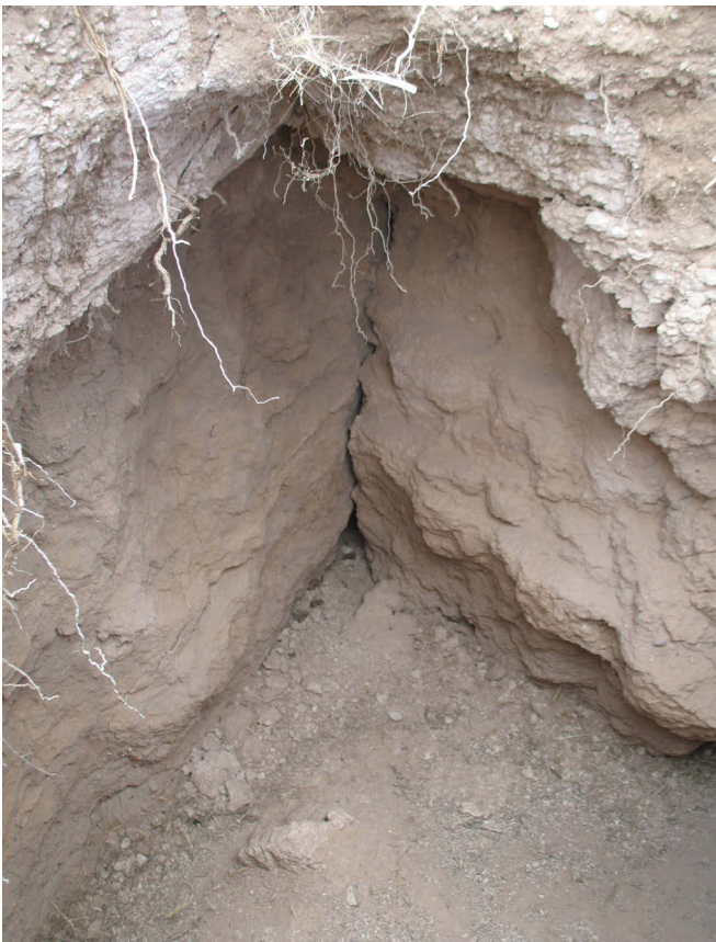
Figure 41. Vertical earth fissure in Cedar Valley exposed in the end of an erosional gully formed along the fissure by infiltration of surface runoff. Photo taken August 2009.
