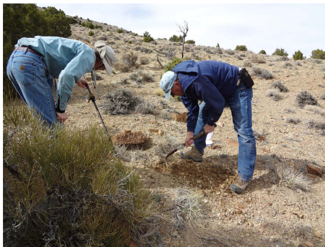
Figure 14. Trenching for fresh samples was often necessary in some portions of recessive units—Jensen Member in this instance; trenching was also essential for accurate surface gamma-ray logging results.
