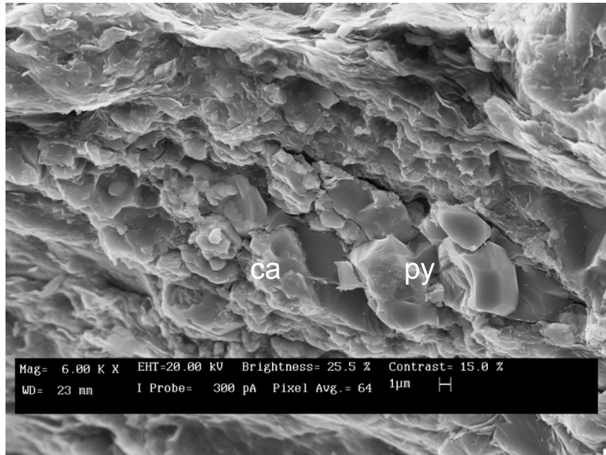
Detailed view showing authigenic cements such as pyrite (py), calcite (ca), and dolomite occluding intercrystalline cavities between layers of clay minerals. (Scale bar = 1 micron)
