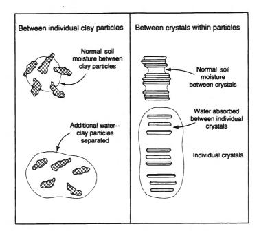
Figure 3. Schematic diagram of water-absorption process in clay minerals.
