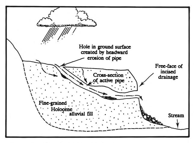
Figure 5. Schematic cross-section of pipe in Holocene alluvium.
