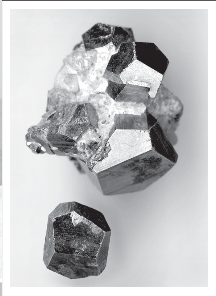
Pyrite crystals commonly form pyritohedrons (twelve irregular five-sided faces) with striations on the crystal faces.
