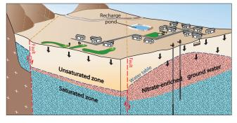
**Figure 7.** Conceptual model of surface-based infiltration. Water is recharged at the recharge pond, infiltrates through an area with a high density of septic systems, creates a recharge mound, and mobilizes nitrate in the previously unsaturated part of the aquifer (Nishikawa and others, 2003).
