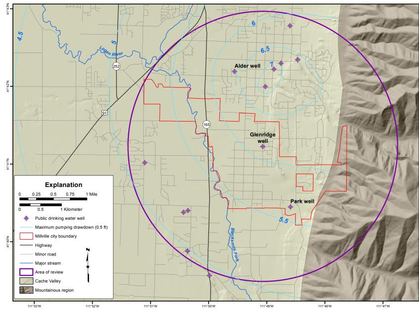
Figure 30. Drawdown contours created using AQTESOLV model of the Millville area. The contours represent maximum pumping conditions, treating the East Cache fault as a barrier to flow. Contour interval is 0.5 feet.
