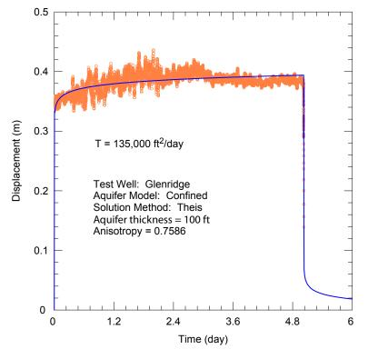
Figure 25. Aquifer test analysis of post-injection pumping data.
