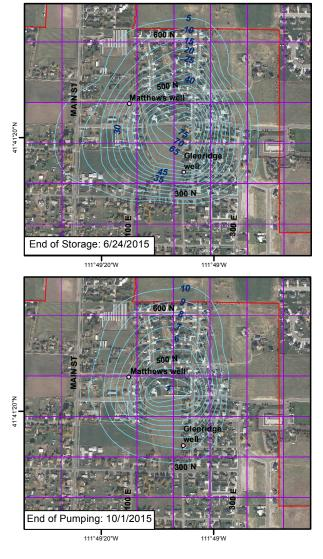
Figure 28. Modeled injectate bubble at different times during phase II. The contours represent percent injectate. Note that the contours are not exactly aligned with the Glenridge well due to offset of the grid cell center from the actual well location.
