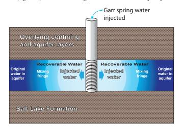
*Figure 4.* Conceptual diagram of storage of injected water in the Cache Valley principal aquifer (modified from Pyne, 1995).
