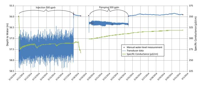
Figure 27. Hydrograph of phase I injection and pumping test of the Glenridge well.
