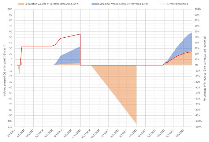
Figure 21. Hydrograph of phase I injection and pumping test of the Glenridge well.
