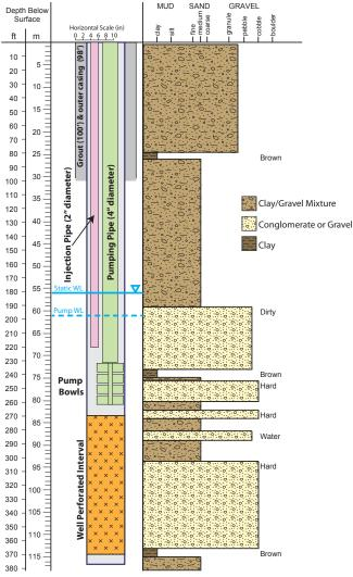
Figure 12. Scale drawing and lithologic record of Glenridge well. Construction data and lithology from appendix B.
