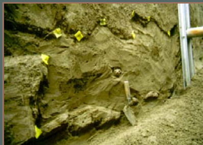
Trench exposure of liquefied sand and disrupted silt interbed.
