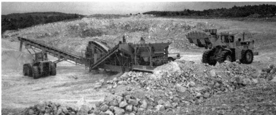
Basin Perlite Company mine showing portable crushing plant, June 1998 (photo credit: North American Exploration).
