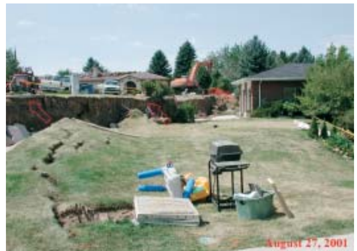
In the left photograph the arrows point to the tilted sidewalk (left) and roll in lawn (right) showing small main-scarp displacements on August 8, 2001. In the right photograph the arrows point to the same locations showing main-scarp displacements of 4 to 5.5 feet on August 27, 2001.
