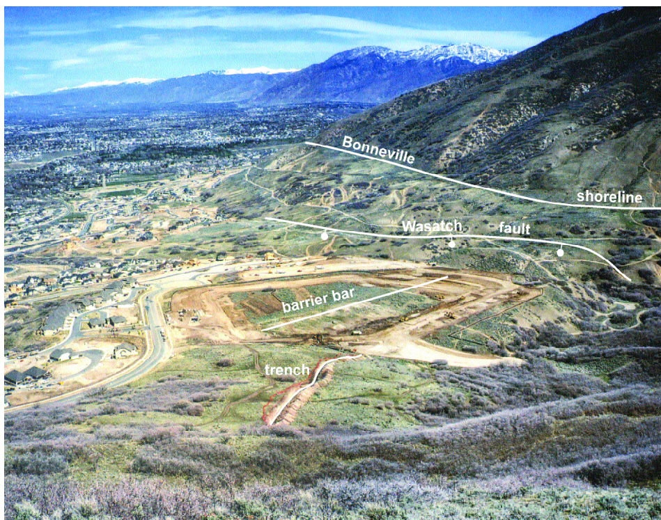
View northeast to the entrance of Corner Canyon. Note the prominent Bonneville shoreline, Bonneville barrier bar, and Wasatch fault scarp (bar and ball on downthrown side). Trench in the foreground was dug to investigate the "Potato Hill" landslide, which overrode the Bonneville shoreline sometime after the lake receded from its highest level.
