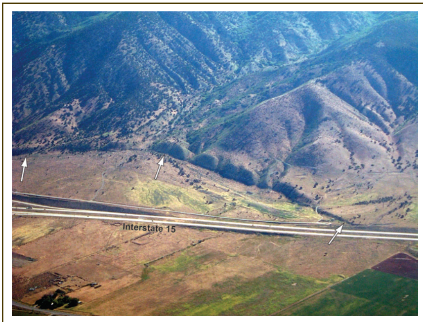
Low-sun-angle oblique aerial photograph of youthful fault scarps (marked by white arrows) near the south end of the Nephi segment of the WFZ. View is to the east. Photo courtesy of Ronald Bruhn (University of Utah).
