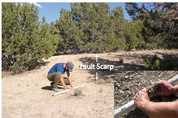
UGS geologist Chris DuRoss measures a profile across a small scarp on the Levan segment. Distance and slope angle are measured using a telescoping stadia rod and Abney level, respectively.
