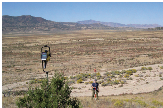
Profile measurements on large scarps were facilitated by use of a laser range finder (above the shrub) and reflecting prism (held by DuRoss). View from near the top of a large scarp on the Fayette segment, looking northwest across northern Sevier Valley to the Valley Mountains (Canyon Mountains in far distance).
