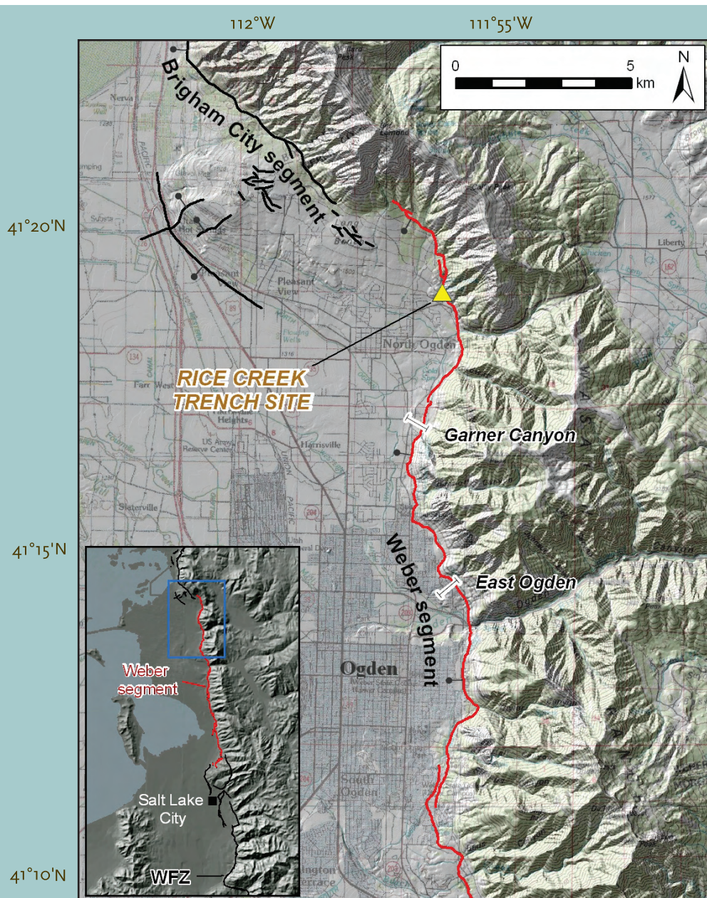
Northern Weber segment of the Wasatch fault zone (WFZ), showing locations of the Rice Creek trench site and previous trench investigations ("I" shapes). Red line indicates trace of the Weber segment; ball and bar on downthrown side.
