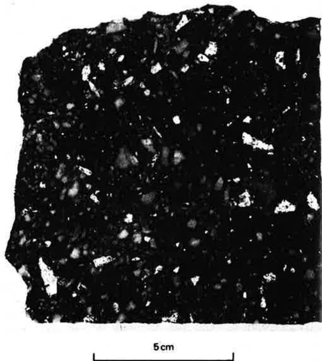
FIGURE 21. — Polished slab of silicified pebble dike from exposure 775 ft (236 m) southeast of Hidden Treasure Spring. White areas are kaolinized fragments of shale from Ophir Formation.
