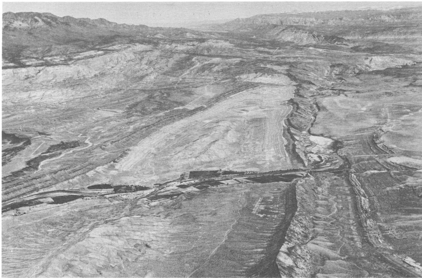
Figure 98. The northeast-plunging Virgin anticline, looking northeast. Note the "corner" in the right middle distance where the projection of the Laramide anticlinal fold is cut obliquely by the later north-south Hurricane fault, the trace of which is marked by the low saddle in the middle distance. The highlands (Kolob Plateau) in the upper right are east of the Hurricane fault. (Photograph by J. R. Shelton and R. C. Frampton.)
