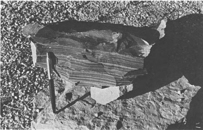
Figure 13. Specimen of rich oil-shale from the Mahogany ledge of the Green River oil-shale beds. Note the characteristic thin black laminations and massive appearance. As a general rule, the richer oil-shales are more black, while the leaner oil-shales grade into shades of brown (Specimen courtesy of G. E. and B. R. Untermann).
