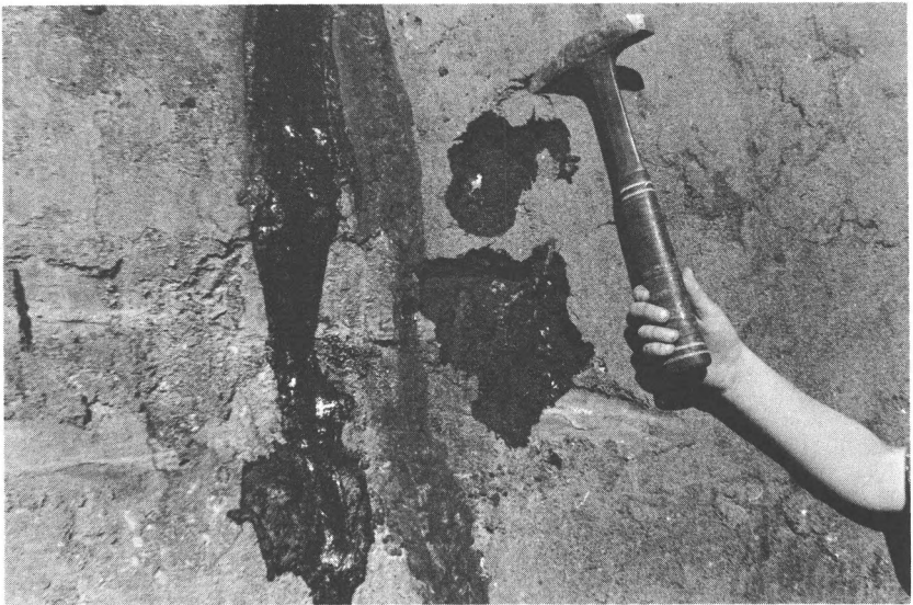
Figure 5. Closeup of the quarry face at the County Asphalt Pit, showing the viscous liquid bitumen, the rich fresh bituminous sandstone (which here is little more than a bituminous cemented sand), and the light gray weathered surface.
