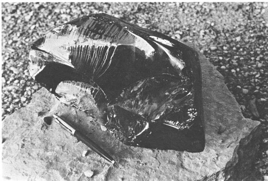
Figure 6. Specimen of "select" gilsonite showing the distinctive conchoidal fractures and vitreous luster. Gilsonite is soft and brittle, and melts at 250-450 degrees Fahrenheit. When exposed to sunlight and atmospheric conditions, gilsonite will become dull and develop minute cracks, gradually breaking down to become "seconds," or more hackly, refractory gilsonite. (Specimen courtesy of G. E. and E. R. Untermann.)
