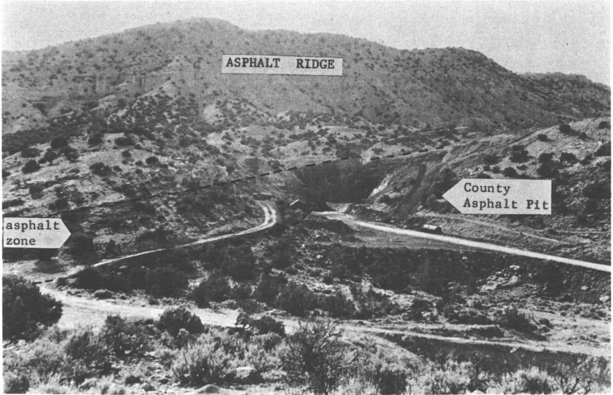
Figure 2. View of the County Asphalt Pit on Asphalt Ridge, looking northwest. This pit has furnished much of the paving material in Uintah County, and is the site of the richest bituminous deposit on Asphalt Ridge. In this picture the bituminous beds dip 10 degrees to the west and underlie the ridge. The bituminous sandstone beds are exposed along the scarp slope of Asphalt Ridge for a length of 12½ miles.
