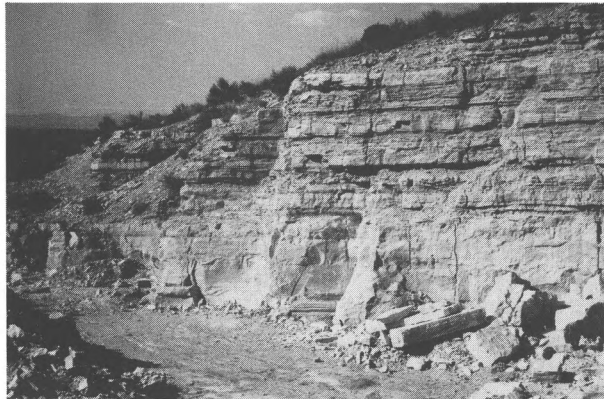
Figure 12. Green River Limestone quarry on Temple Hill near Manti. The 8-foot oolite bed at base of quarry is used for building stone.
