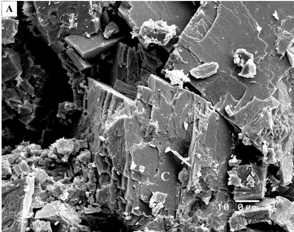
Photomicrograph 3A. Lisbon B-610. SEM photomicrograph of a core plug from 7886'. Enlargement showing rare calcite cement (C). Black is porosity. Scale represents 10 microns (0.01 mm).
