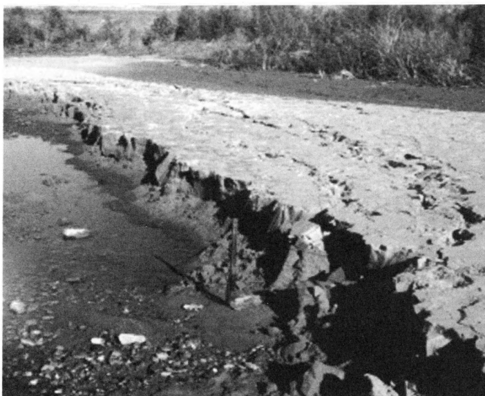
Figure 12. Lateral-spread cracking from liquefaction along the Virgin River. Photo by W.E. Mulvey.
