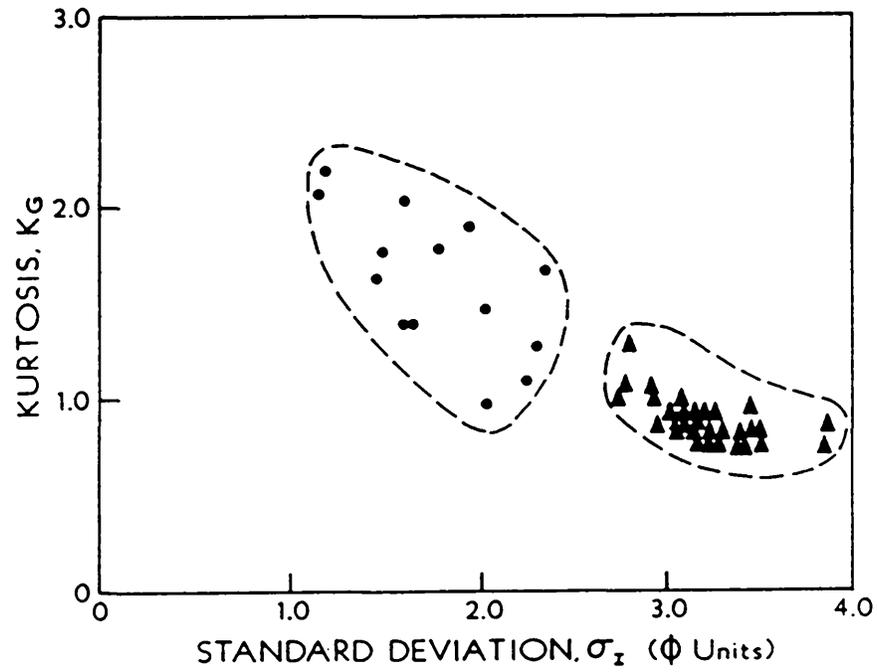
Figure 12. Scatter plot of kurtosis versus standard deviation showing distinct fields for debris-flow (triangles) and hyperconcentrated flood (circles) deposits.
