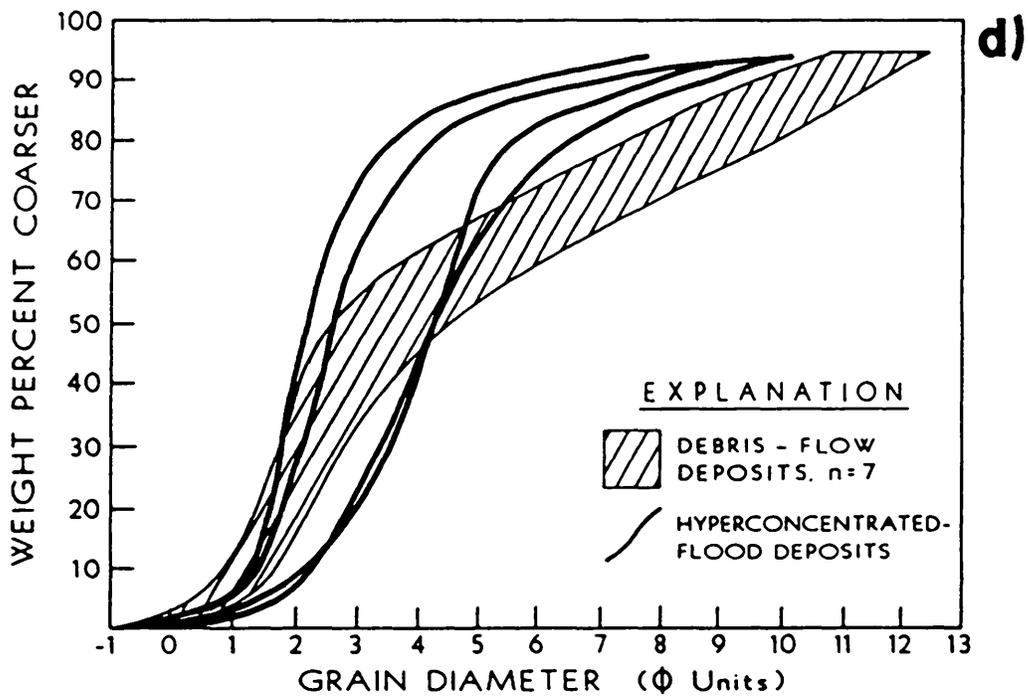
Figure 9. Grain-size distribution curves of the matrix from c) the Lower Gooseberry Reservoir-I debris flow, and d) the Lower Gooseberry Reservoir-II debris flow.
