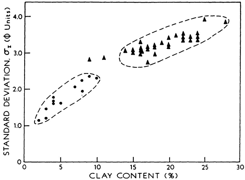
Figure 11. Scatter plot of standard deviation versus clay content showing distinct fields for debris-flow (triangles) and hyperconcentrated-flood (circles) deposits.
