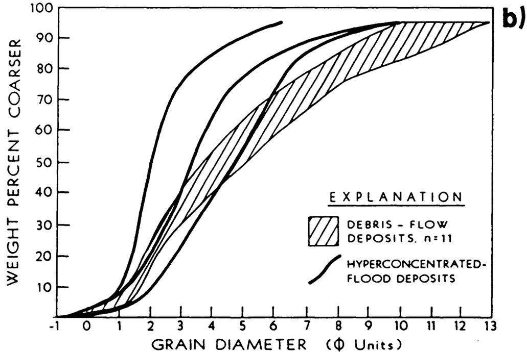
Figure 9. Grain-size distribution curves of the matrix from a) the Birch Creek debris flow, and b) the Crooked Creek debris flow.
