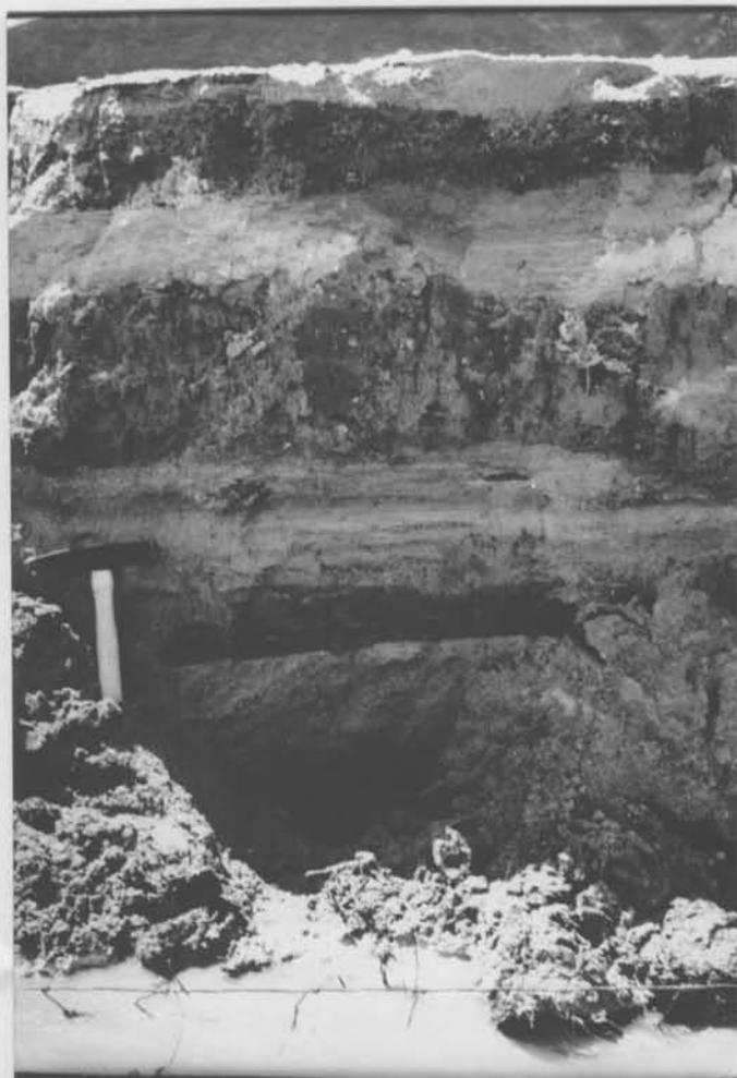
Figure 8. Excavated section of debris-flow deposits (dark layers) and hyperconcentrated-flood deposits (light layers) the Birch Creek debris flow where the flow crossed Utah State Highway 117. The darker-colored deposits were gray, massive, and unsorted consisting of clay to cobble-size material and containing abundant woody debris. The lighter colored deposits were light brown to tan, finely bedded, well-sorted sands containing almost no woody debris.
