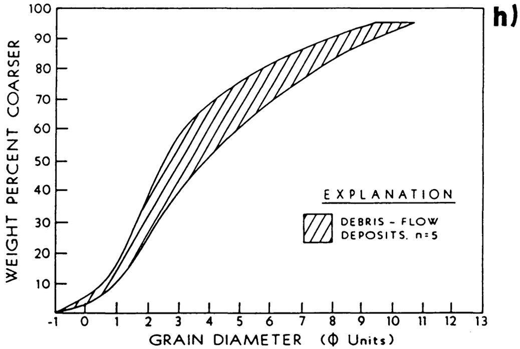
Figure 9. Grain-size distribution curves of the matrix from g) the Pole Canyon debris flow, and h) the Ward Canyon debris flow.
