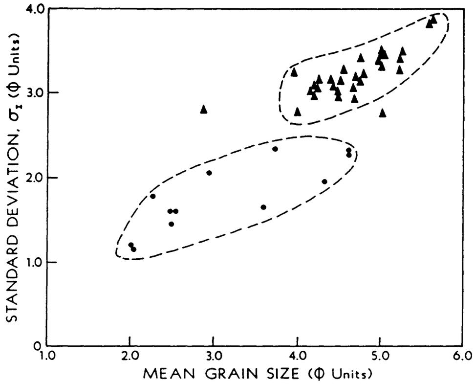
Figure 10. Scatter plot of standard deviation versus mean grain size showing distinct fields for debris-flow (triangle) and hyperconcentrated-flood (circles) deposits.
