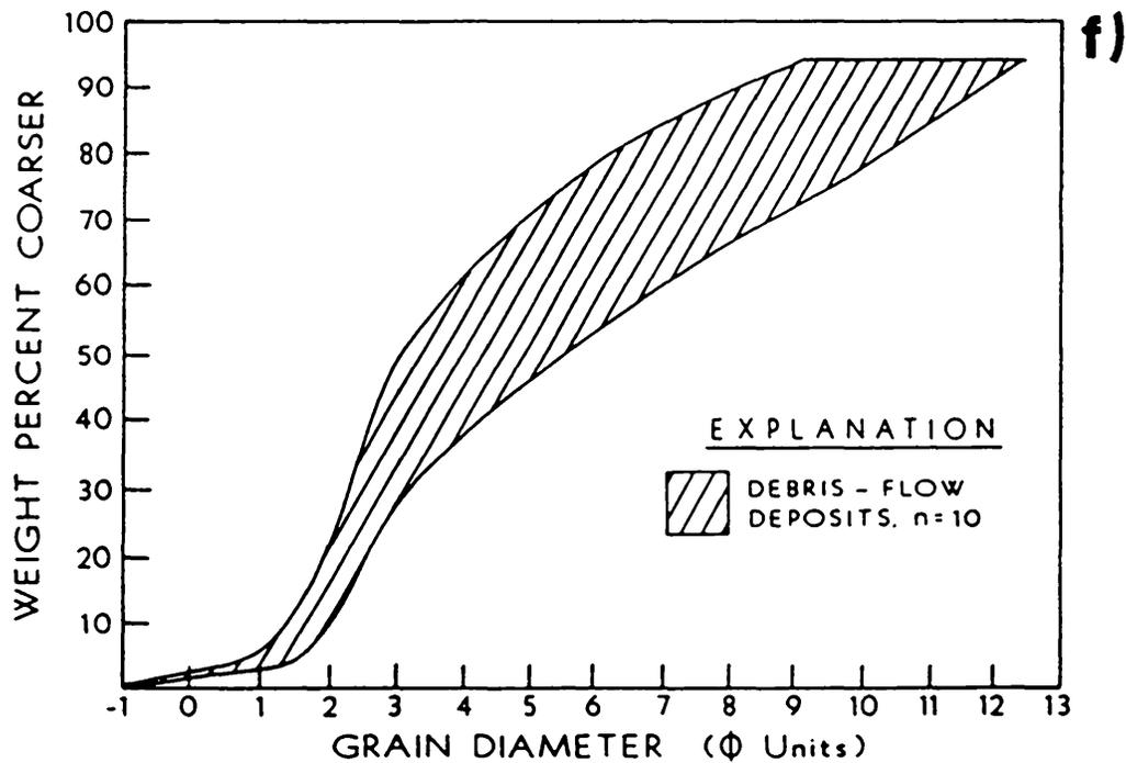
Figure 9. Grain-size distribution curves of the matrix from e) the Little Clear Creek debris flow, and f) the South Fork North Creek debris flow.
