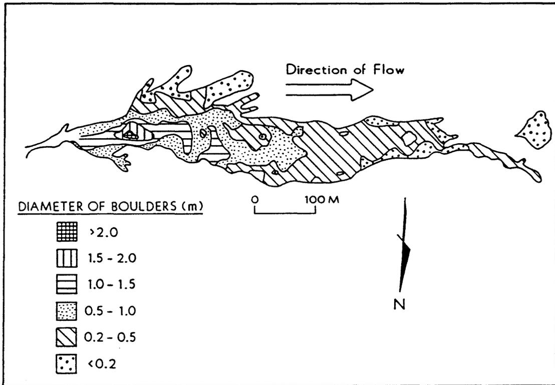
Figure 4. Map showing depositional area of the Lower Gooseberry Reservoir I debris flow showing the distribution of boulders. The largest boulders were concentrated in the center of the deposit and near the canyon mouth. As distance from the canyon mouth increased, the boulders decreased in size.
