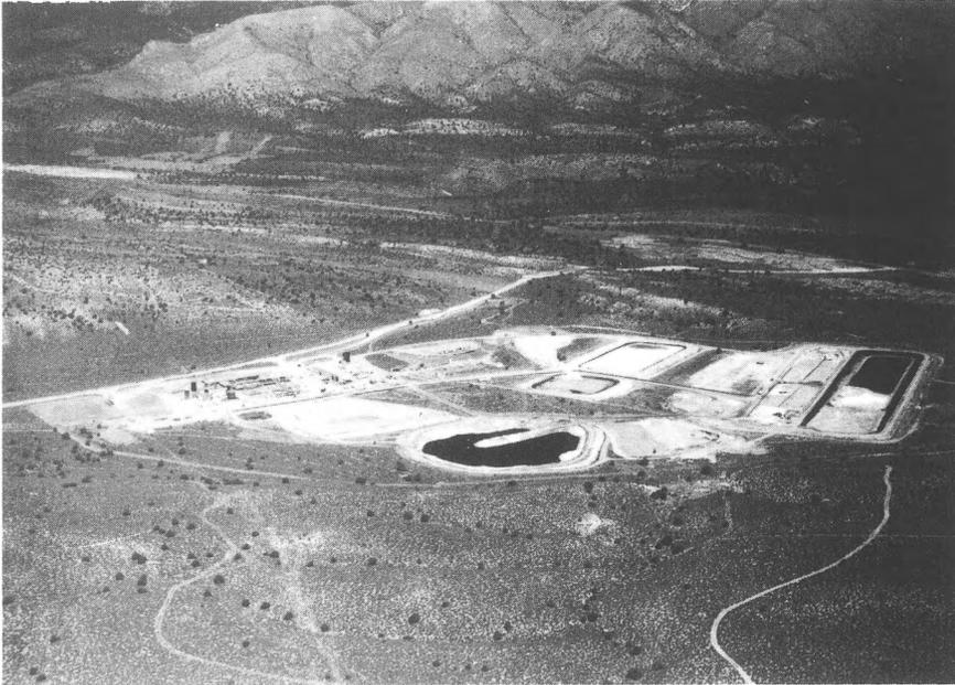
**Figure 10.** Aerial view looking northwestward at the Apex Mill in June 1991. The ponds hold tailings produced in the mill by rock-leaching operations.
