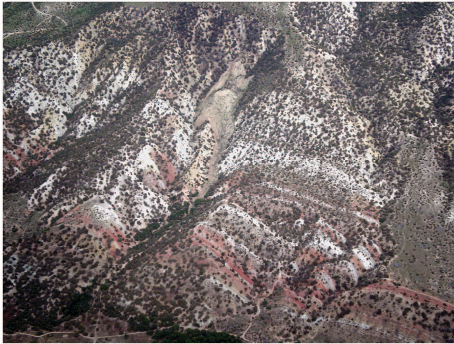
Figure 1. Aerial view of the Colton Formation along the west side of the Wasatch Plateau. The colorful formation dips an average of 45^\circ valleyward in the steepest part of the Wasatch monoclinial structure. Note the landslide in the upper middle part of the photo.
