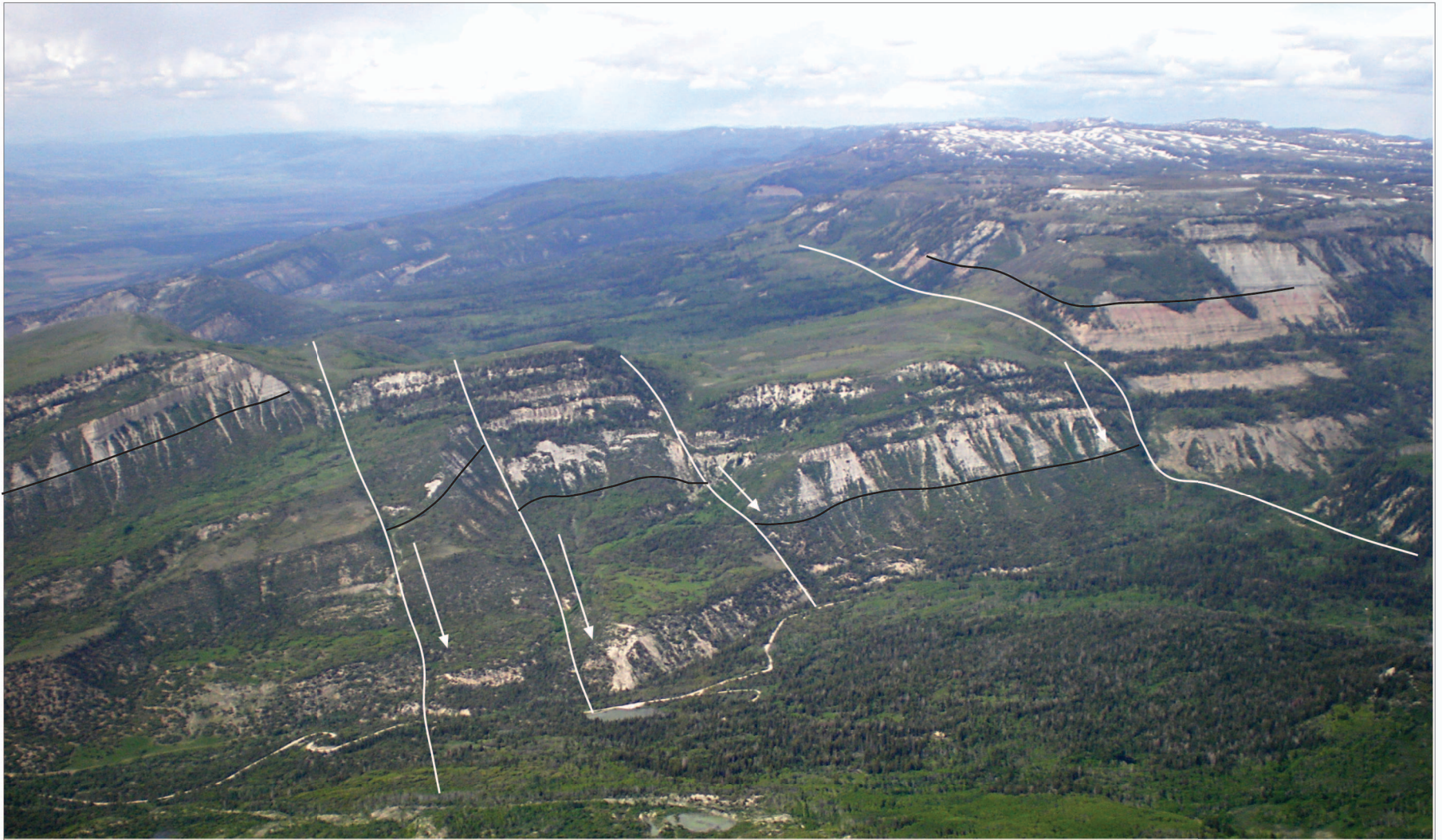
Figure 7. Aerial view northward across Manti Canyon showing downthrown blocks and the Shoulder graben. White lines are the approximate fault traces. White arrows are shown on the side of downward displacement. Black lines mark the approximate boundary between the Flagstaff Limestone (light outcrops) and the North Horn Formation (pink outcrops). Photo also shows the form of the Wasatch monocline.
