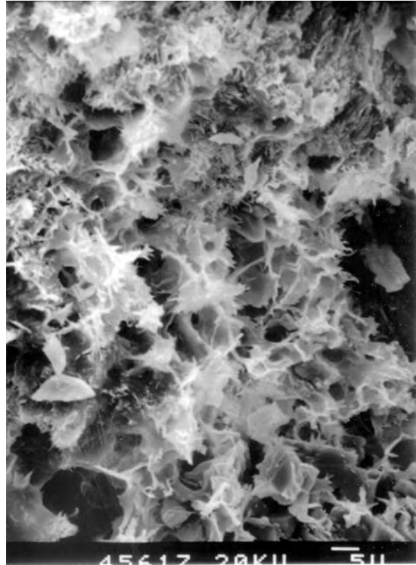
More detailed view of secondary illite and associated micropores. EDX peaks for Si, Al, and K confirm illite composition. Delicate, well-formed illite fibers and flakes are highly susceptible to breakage and migration through the pore system. Concentrations of illite at pore throats can significantly reduce permeability in areas of high flow velocity. Scale bar = 5 microns. (1100 \times )
