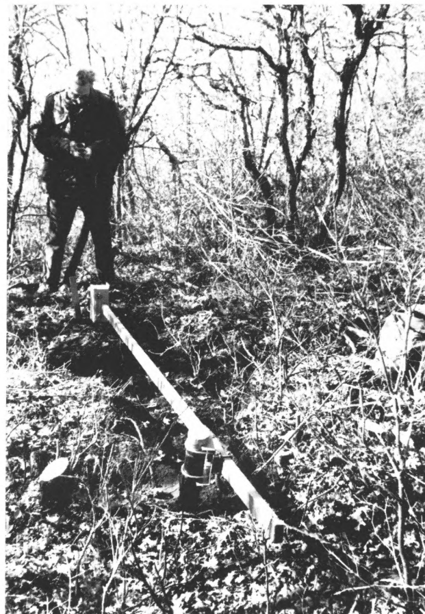
Figure 8. Davis County watershed Left: Appearance of watershed immediately following a debris slide; right: Extensometer installation in Rudd Creek Canyon.
