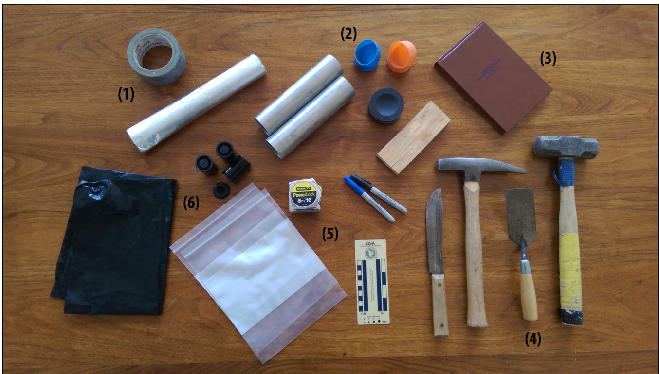
Figure 2. Possible sampling equipment. (1) Duct tape and aluminum foil. (2) Metal tubes and plastic/rubber end caps. (3) Field notebook. (4) Hammers, trowels, and wooden block to hammer against. (5) Measuring tape, permanent markers, photo scale, zip-locking bags. (6) Film canisters and light-proof bag. Light-proof bags can be obtained from a photography supply store.
