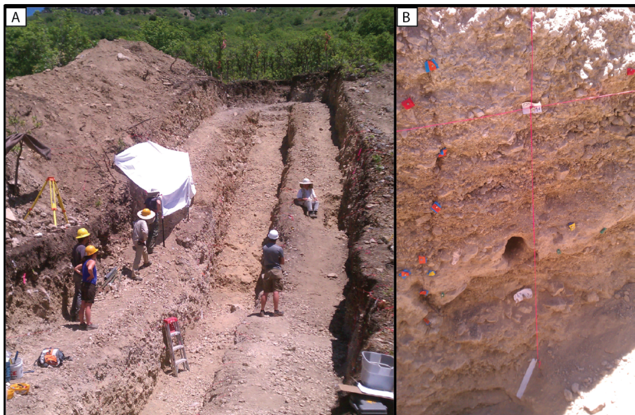
Figure 1. (A) Typical paleoseismic trench in a coarse alluvial-fan setting. (B) Example luminescence age sampling location on the trench wall. Note the sample is in a sandy layer between coarse, poorly sorted layers. Sample site hole is approximately 15 cm in diameter. Hole is larger than tube used for sampling.
