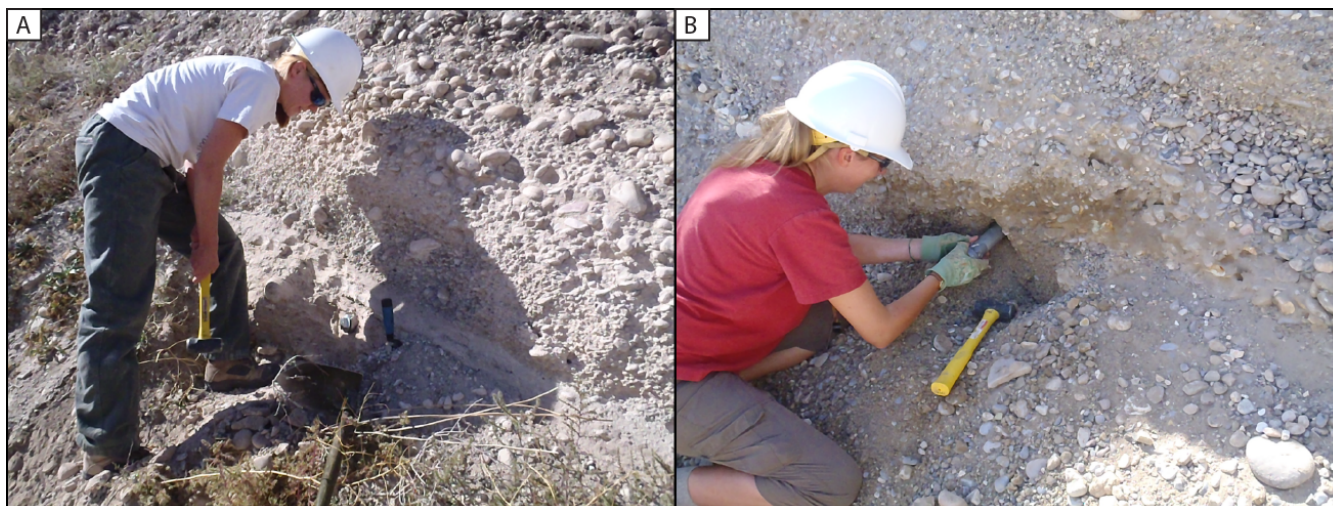
Figure 3. (A) Example of tube collection of finer grained layer between moderately cemented coarse sediments. See text for detailed instruction. (B) After pounding into the outcrop, the tube is carefully extracted without allowing material to shift or fall out of the tube. The next steps are to collect a dose-rate sample, a sample for water content, measure the depth of the tube to the above surface, and to document the sample location (latitude, longitude, and elevation) and nearby sedimentology.
