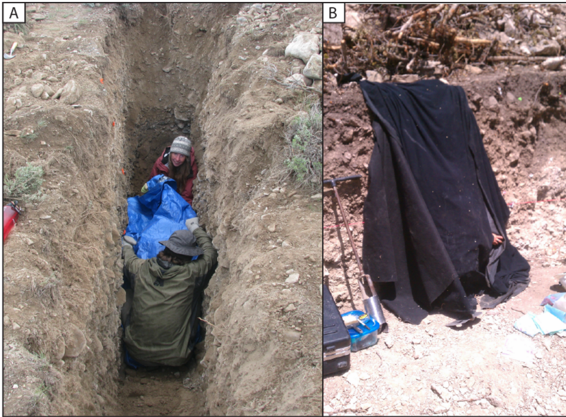
Figure 4. (A) Example of canister collection. Here two individuals assist the sampling by draping an opaque tarp over the sample location as the finer grained matrix material is collected from around large clasts and immediately placed into a light-proof container. (B) In some instances, a dark blankets can be held in place on its own.
