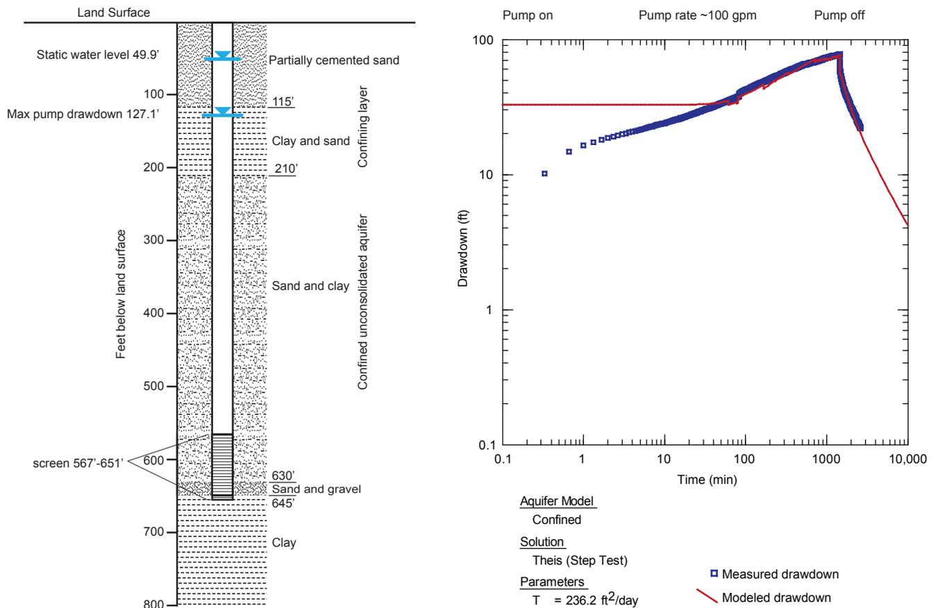
Figure 15. Well log and aquifer test solution for well FWW.
