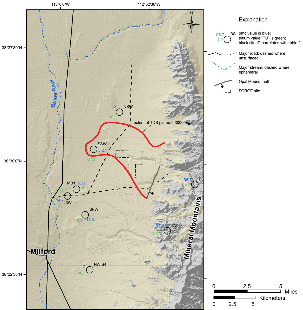
**Figure 11.** Map of carbon isotope and tritium samples. Isotopic compositions typical of recharge are shown at sites KS and BS. Samples near the high-TDS plume have low pmc and tritium values.
