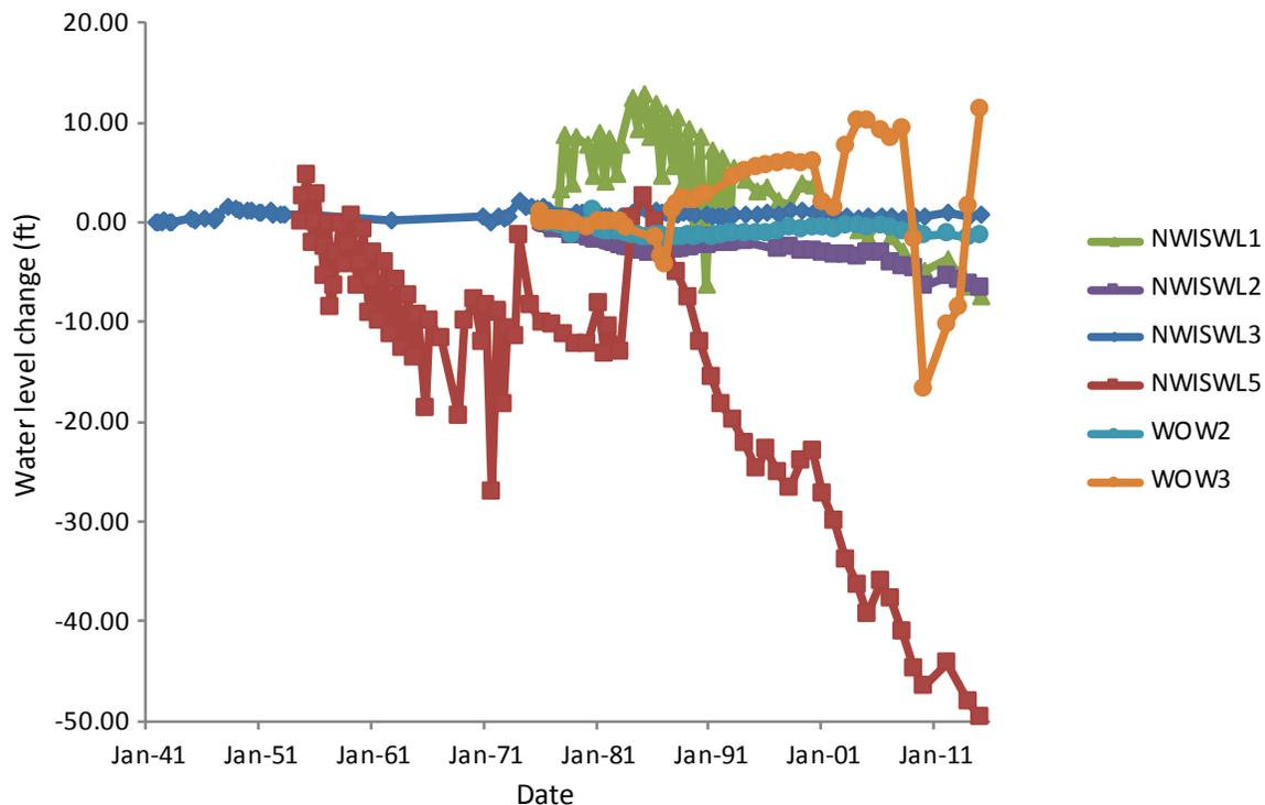
**Figure 4.** Long-term water level changes in groundwater wells. Data used to construct the graph are from the USGS NWIS database (U.S. Geological Survey, 2017). Long-term water level changes near the FORGE deep drill site are less than 10 feet. To the south, near Milford, NWISWL5 shows a decline of 50 feet from 1985 to present, which is interpreted to be due to agricultural groundwater use.
