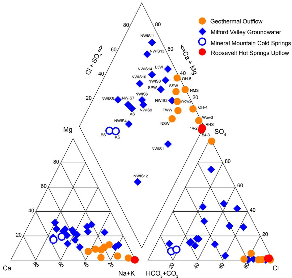
Figure 6. Piper diagram of compiled groundwater chemistry. Site ID corresponds with those in Table 2.
