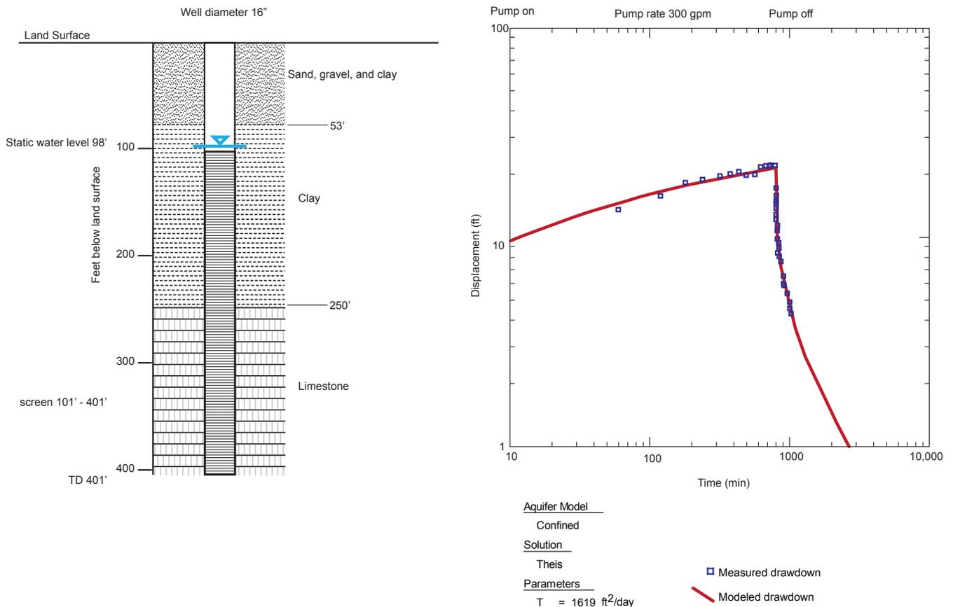
Figure 14. Well log and aquifer test solution for well MBW-2.
