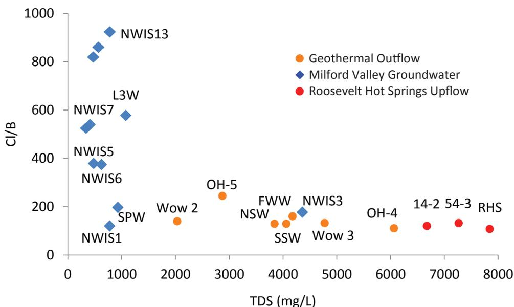
**Figure 8.** Graph of Cl/B versus TDS. Most groundwater samples surrounding the FORGE deep drill site have uniform Cl/B values of ~150 with decreasing TDS resulting from mixing and dilution.
