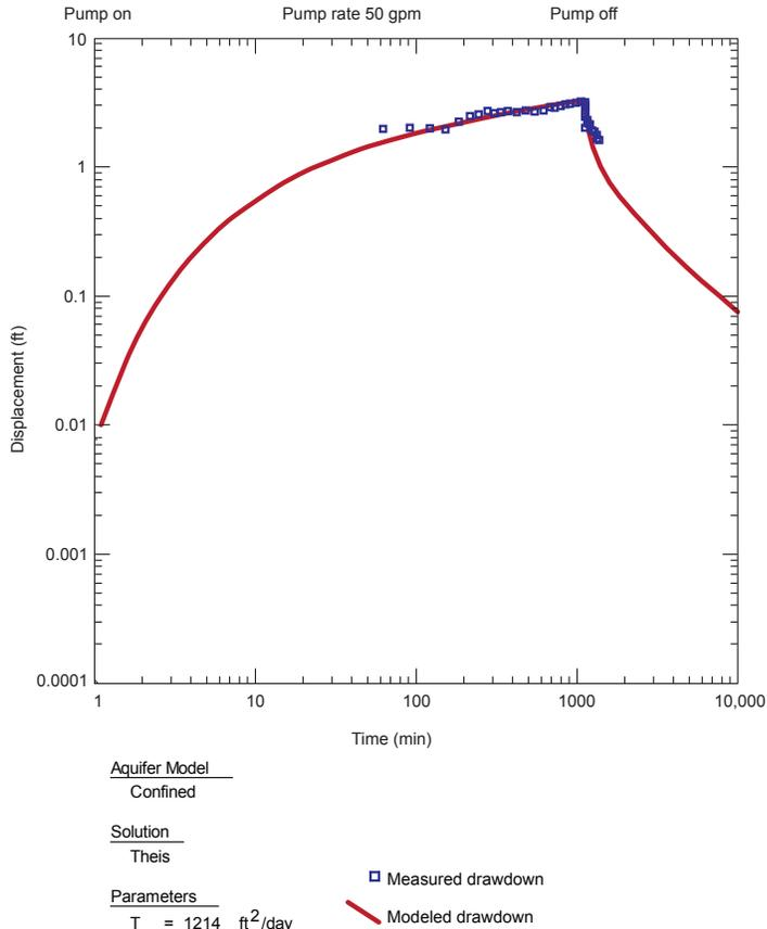
**Figure 13.** Well log and aquifer test solution for well MBW-1.
