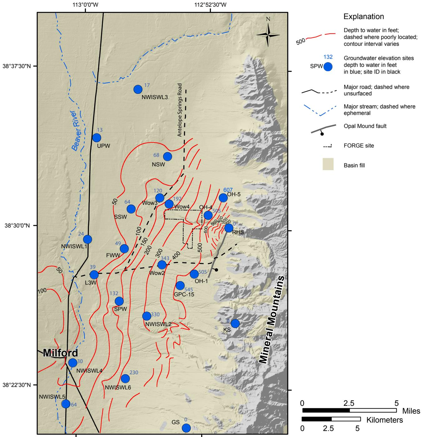
**Figure 3.** Depth-to-water map for the FORGE study area. Depth to water calculated as the difference between the potentiometric surface in Figure 2 and a 5-meter digital elevation model.
