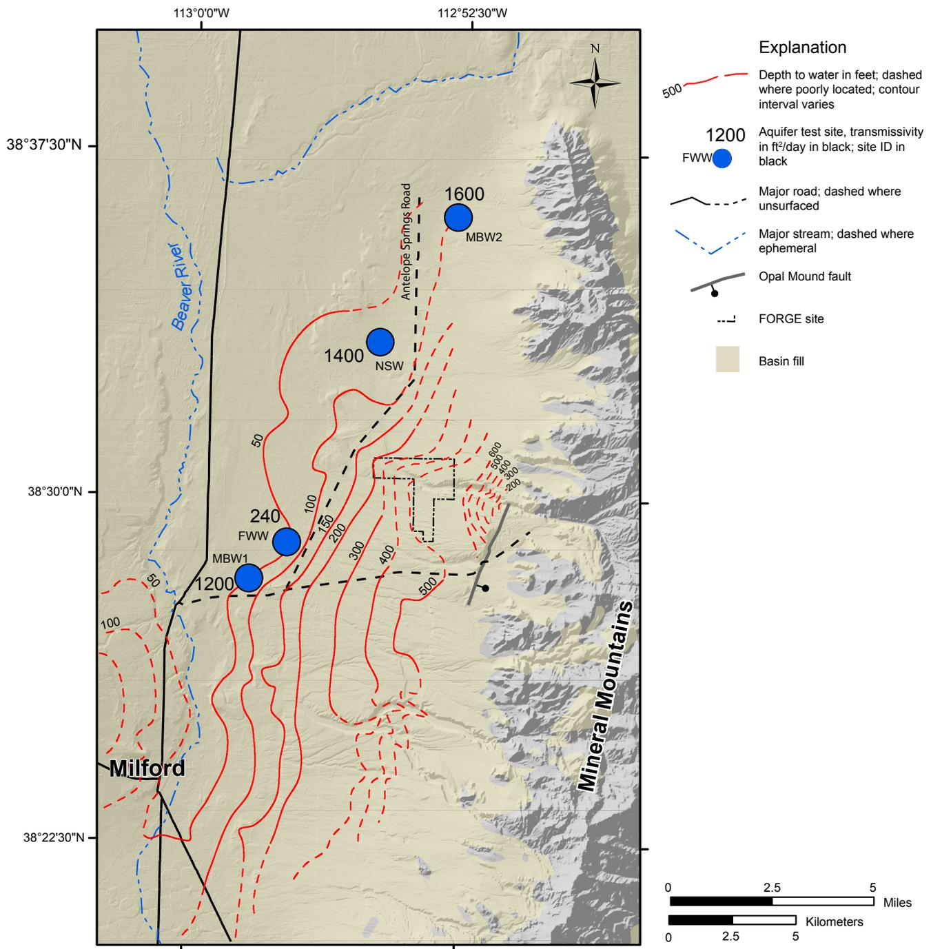
**Figure 16.** Summary of aquifer test data for the basin fill aquifer. Transmissivity of the basin-fill near the FORGE site ranges from 240 to 1600 ft<sup>2</sup>/day.
