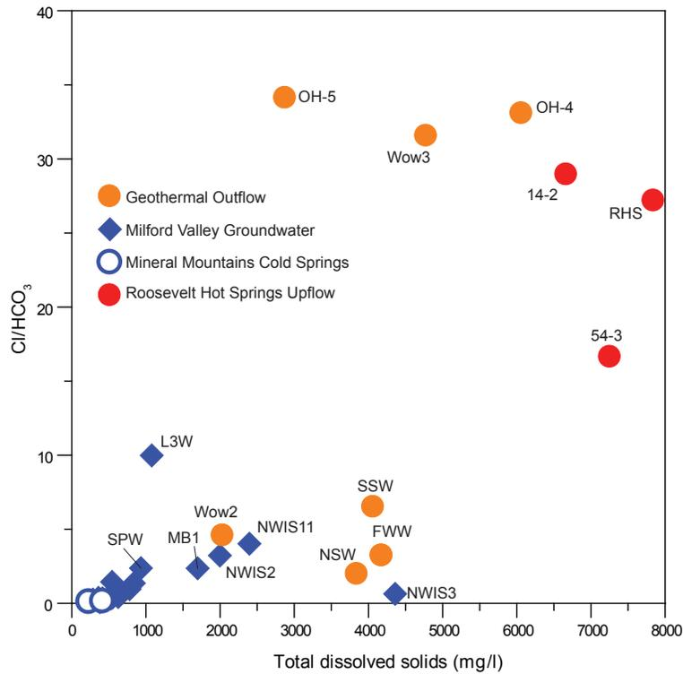
Figure 7. Graph of the ratio of Cl and HCO<sub>3</sub> anions versus total dissolved solids. Samples do not lie along a simple mixing trend, implying that simple end member mixing does not control all chemical variation.
