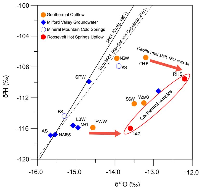
**Figure 10.** Plot of stable isotope compositions (per mil) of groundwater. The meteoric water line (MWL) is defined by Craig (1961) and the Utah meteoric water line is defined by Kendall and Copeland (2001). Thermal water (14-2 and RHS) shows a significant positive shift in  $\delta^{18}\text{O}$  relative to local meteoric water due to isotope exchange during high-temperature water-rock interaction.
