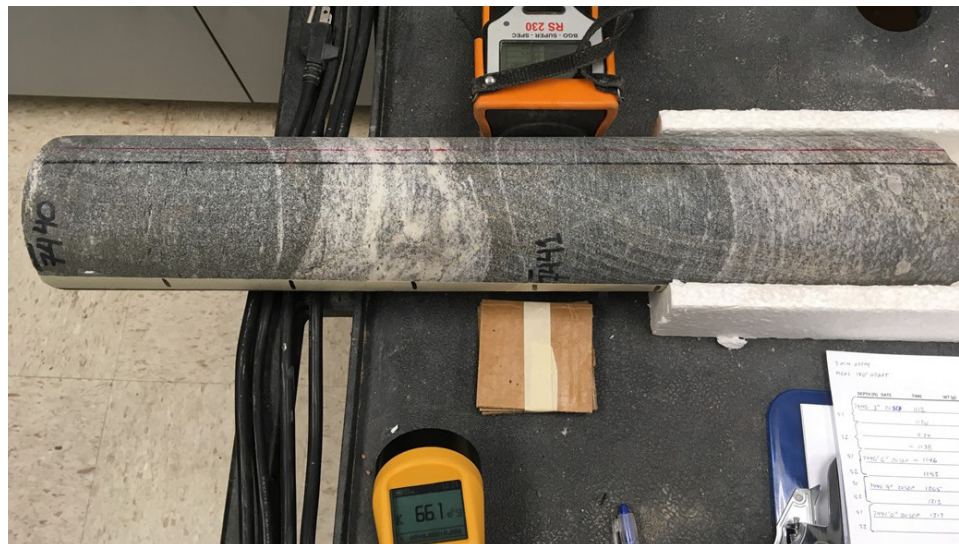
Figure 23. The RS-230 Gamma Ray Spectrometer (top center of photograph) in use on the lower core section (top at 7440 feet). Spectral gamma ray measurements were made at 3-inch intervals along the entire length of the reconstructed core. A second measurement was made on the opposite side of the core at each depth. The yellow instrument at the bottom of the photograph is the KT-10 Magnetic Susceptibility Meter that was used at the same measurement locations as the spectrometer.
