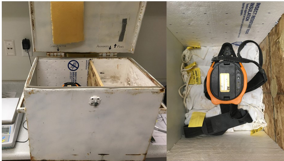
Figure 22. The RS-230 Gamma Ray Spectrometer in use on cuttings from well 58-32. Spectral gamma ray measurements were focused at 100-foot intervals, but due to limited sample mass, additional samples from above and below the target depth were needed to achieve a minimum mass experimentally determined from outcrop samples. Therefore, measurements were made using samples from an 80-foot interval with the spectrometer positioned over the targeted sample (photo on the right) so that the greater part of the gamma signal comes from the target depth. Measurements were made in a 5-mm-thick steel box (photo on the left) to attenuate a portion of the background gamma signal.
