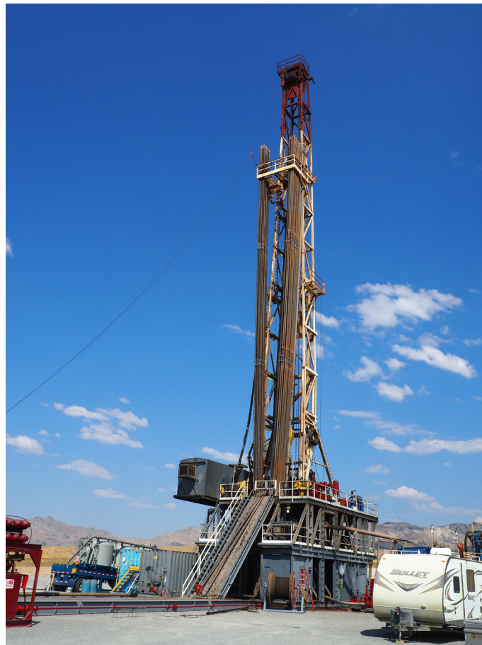
Figure 2. Kenai Rig 10 on the 58-32 well pad. Photograph taken on September 3, 2017, during the running of temperature logs at an intermediate depth of 6800 feet.
