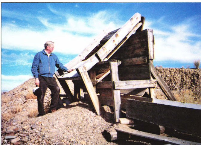
Gravel screening device and sluice box used for gold concentration along the Green River.
