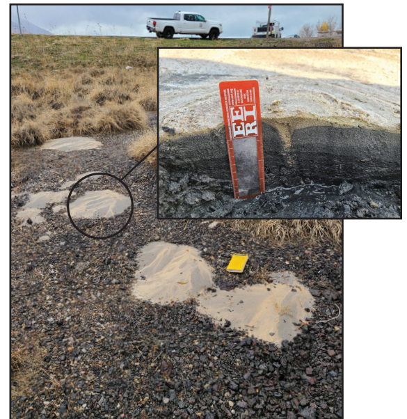
Sand boils near the Great Saltair event center caused by ground-shaking-induced liquefaction from the Magma earthquake. Photo courtesy of the Utah Geological Survey.
