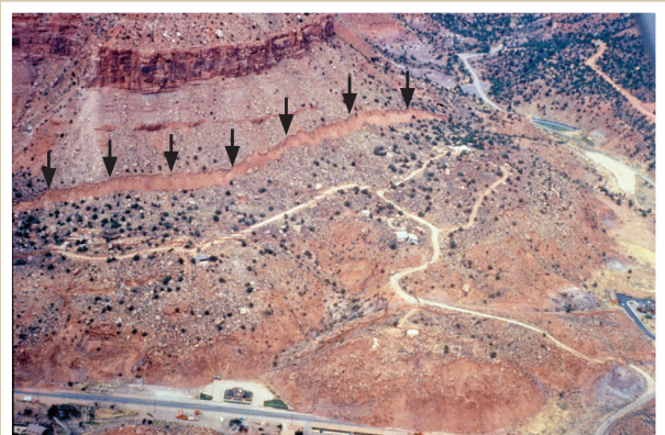
Aerial view of the Springdale landslide, triggered by the September 2, 1992, M 5.5 St. George earthquake. The top of the landslide is denoted by black arrows. Photo courtesy of the Utah Geological Survey.
