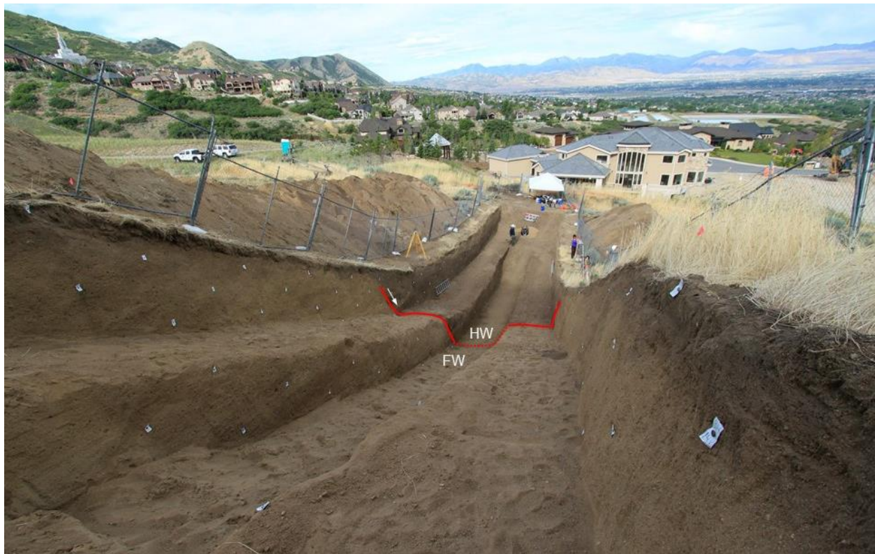
Figure 5. Photo of the Corner Canyon trench. Fault zone shown in red with hanging wall (HW) and footwall (FW) annotated. Arrow shows direction of movement on fault. Photo direction is SW. Photo taken on June 22, 2014.
