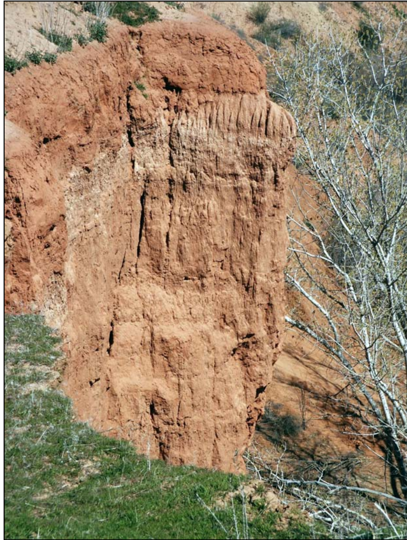
Figure 5. Vertical cracks parallel to the arroyo wall in an area adjacent to the landslide that has not yet failed; such cracks are typical where arroyo walls are vertical.
