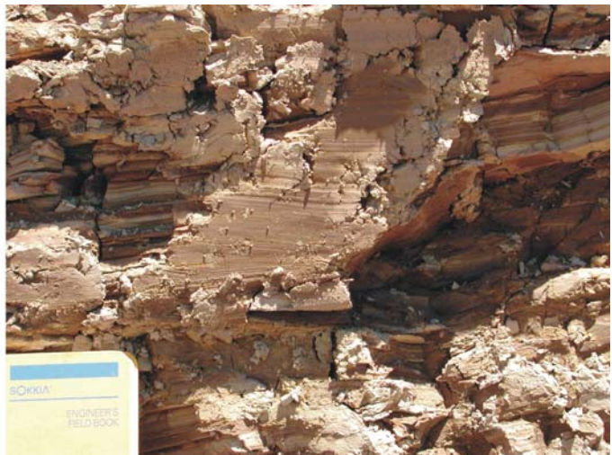
Figure 5. Exposure of laminated lacustrine clay south of the Frontier Drive landslide. Field book shown for scale.
