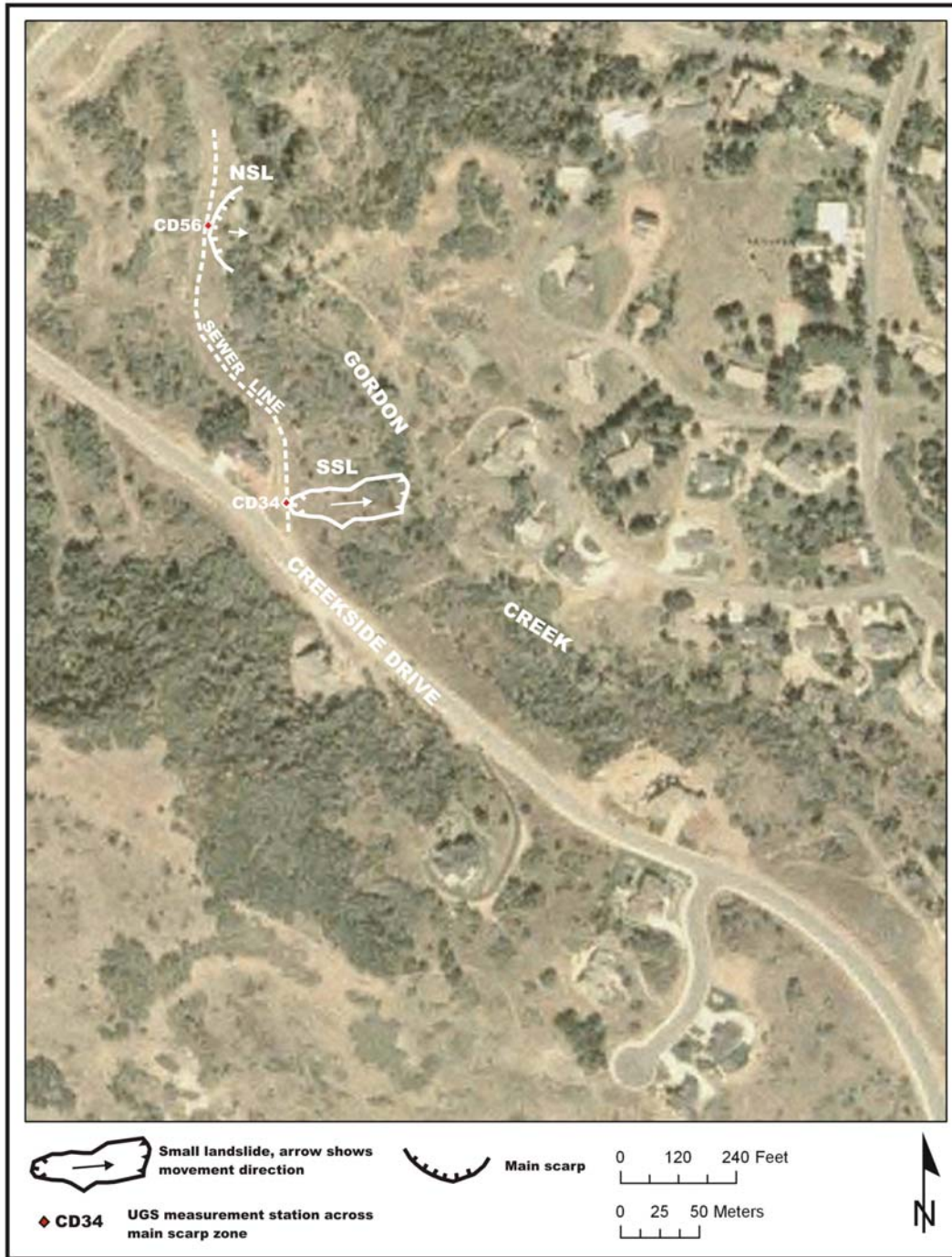
Figure 2. Aerial photograph showing approximate locations of two small landslides between Gordon Creek and buried sewer line northeast of Creekside Drive in Mountain Green. Northern Sewer-Line (NSL) and Southern Sewer-Line (SSL) landslides shown. Locations and boundaries of landslides approximate.
