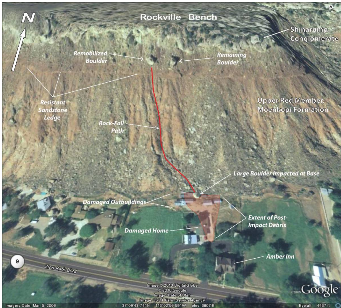
Figure 2. Google Earth image showing source area, rock-fall path, extent of post-impact debris field, and damaged structures.
