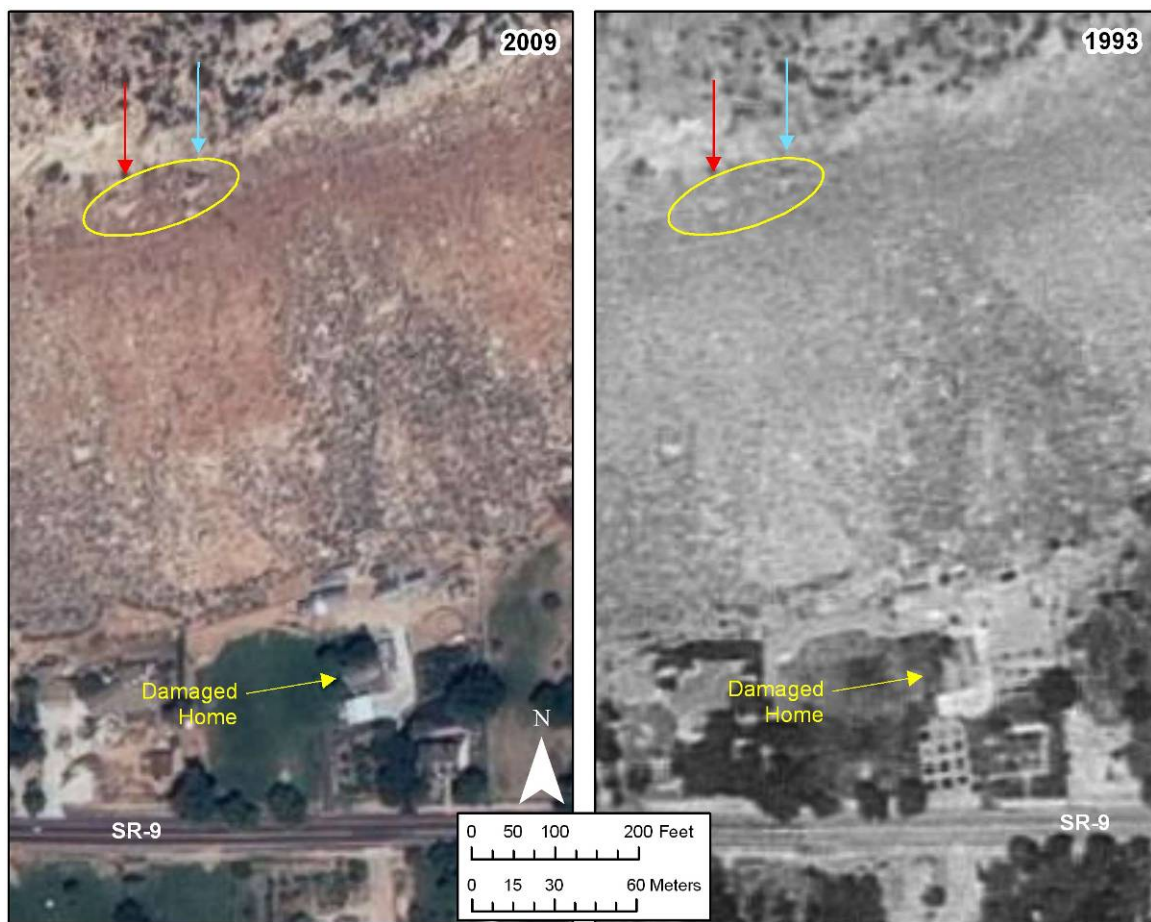
Figure 5. Comparison of 2009 NAIP and 1993 U.S. Geological Survey orthophotos showing the source area and damaged home. Both the 2010 rock fall (red arrow) and the boulder remaining on the hillside (blue arrow) are visible in the 2009 photo; although not as clear, the boulder pair also appears to be present in the 1993 photo.
