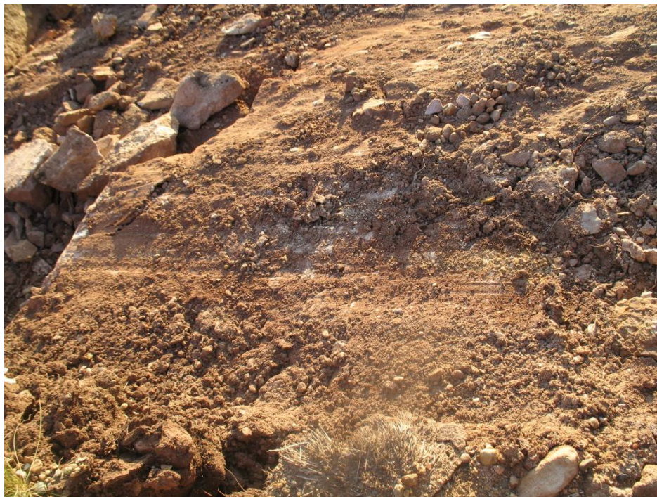
Figure 6. Slide plane and grooves (~5 feet long) in the detachment area; left is downslope.
