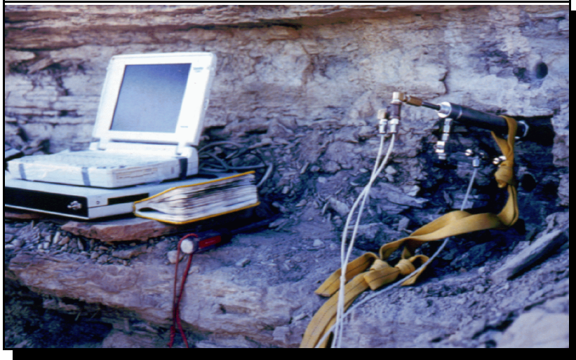
Figure 6. The electronic miniprobe permeameter measuring permeability in a core hole in the Ivie Creek area.
