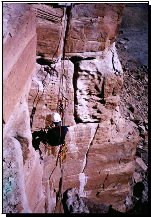
Figure 5. Core-plug sampling along a vertical permeability transect in the Ivie Creek area.
