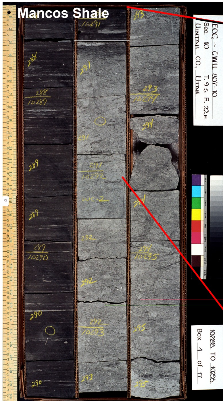
Figure 34. Core photo of 8 ft of section near the contact between the Blackhawk “A” Sandstone and overlying dark-gray marine shales.
