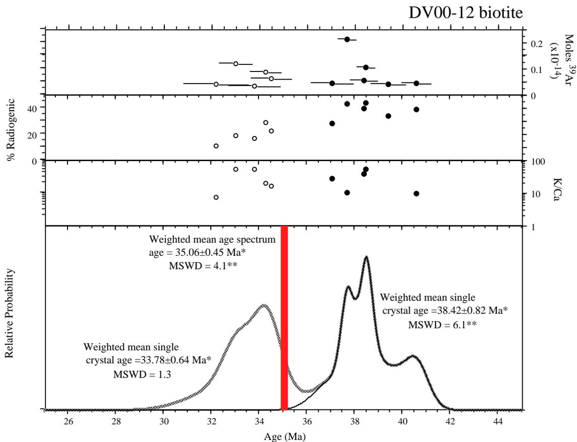
Figure 6. Age probability distribution diagram of b steps for sample DV00-12 single crystal biotite. Red bar indicates weighted mean age calculated from bulk step-heating analysis. \*2 error \*\*outside 95% confidence interval
