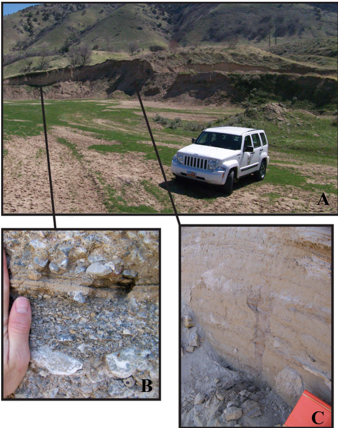
Figure 20. Photographs of Providence sand pits. A. Pit area looking east. B. Close-up view of gravel lens. C. Close-up view of fine sandy material.
