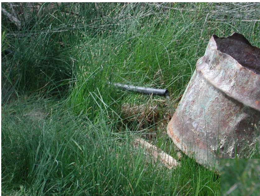
Figure C.3. Site 5. Park-USGS shows capped well and hose leading from well head to pond; samples were obtained from the pipe.
