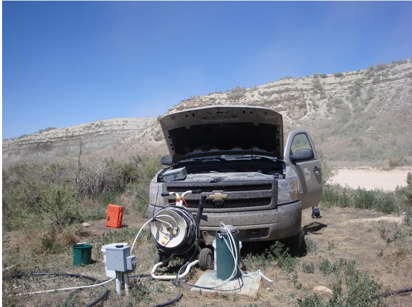
Figure C.4. Site 6: Kings well located in the central part of the study area is along King's Well Road; a battery powered submersible Hurricane Pump was used to sample and bail this well three times the volume of the well.
