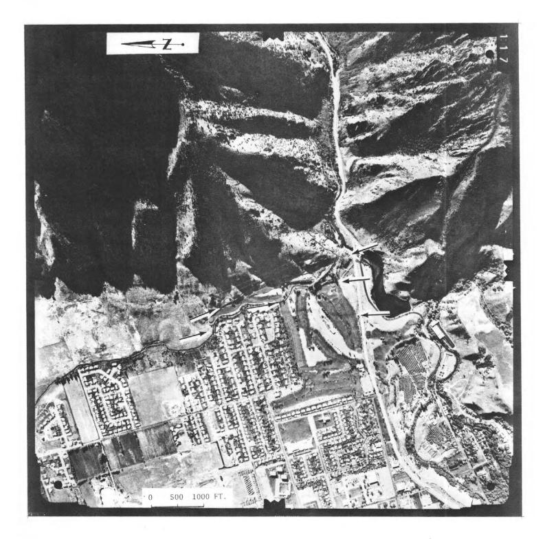
FIGURE 21. Vertical aerial photograph of the East Cache fault at Logan, Utah. The view is southeast. Active traces of the fault are between, but not limited to, the area between the arrows. The fault scarps show as lines of shadows, especially through the Golf Course. See also Figures 22 and 23 and the cover photograph.
