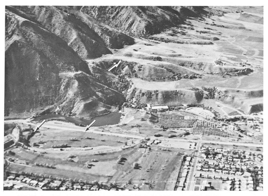
FIGURE 22. Oblique aerial photograph of the East Cache fault at Logan, Utah. Stream erosion in Logan Canyon has removed recent evidence of faulting in the Canyon. Some of the recently active fault traces are indicated by arrows. See also Figures 21 and 23, and the cover photograph.
