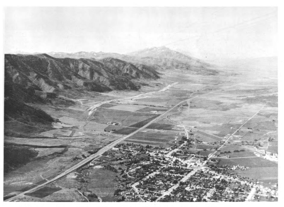
FIGURE 15. Oblique aerial photograph of the Wasatch fault at Malad, Idaho. The view looks south-southeast, Malad is in the foreground. The most recent faulting this area is along the base of the Malad Range, but because it is subdued, it is inferred to be relatively older than the most recent surface faulting in the area of Salt Lake City.
