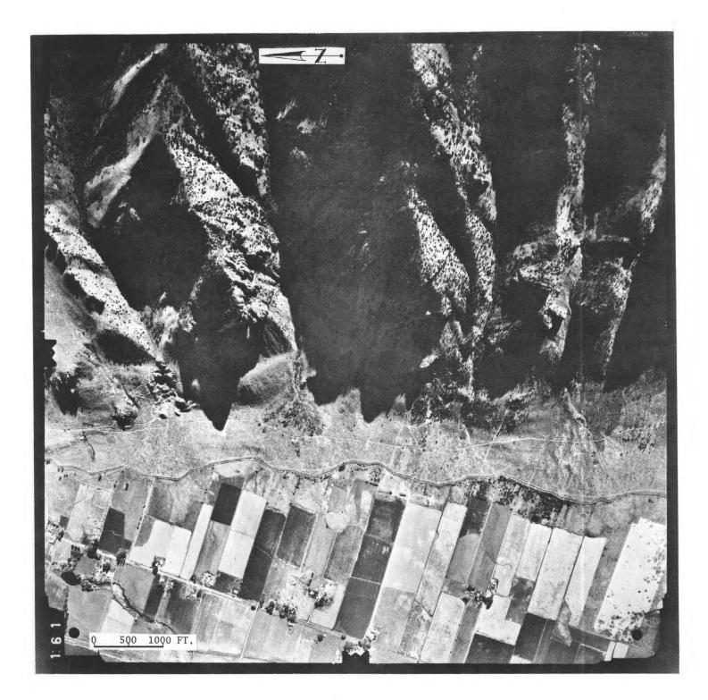
FIGURE 8. The Wasatch fault near Deweyville, Utah. This Low-Sun-Angle Aerial photograph shows the narrow alluvial apron between the cultivated fields and the range front. The cultivated area appears to have been tilted toward the range by faulting, yet the most recent fault scarps are either buried by the alluvial apron or are old and subdued within it.
