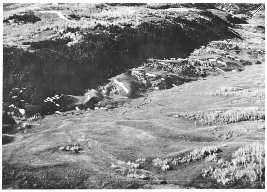
FIGURE 5. Active fault southeast of Logan, Utah. A view of this low oblique aerial photograph is southwest of Bear Lake, in the area of Saddle Creek. This fault, indicated by arrows, is one of several active faults in that area, which is outside of the limits of this investigation.
