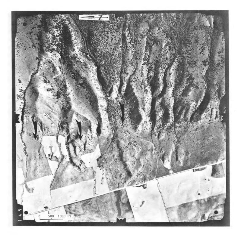
FIGURE 14. Vertical aerial photograph of Clarkston Mountain. This view of the southwest range front shows numerous large landslides that may have been triggered by earthquakes. The most recent active trace of the Wasatch fault in this area is along the base of the mountains and does not appear to displace any of the landslides.
