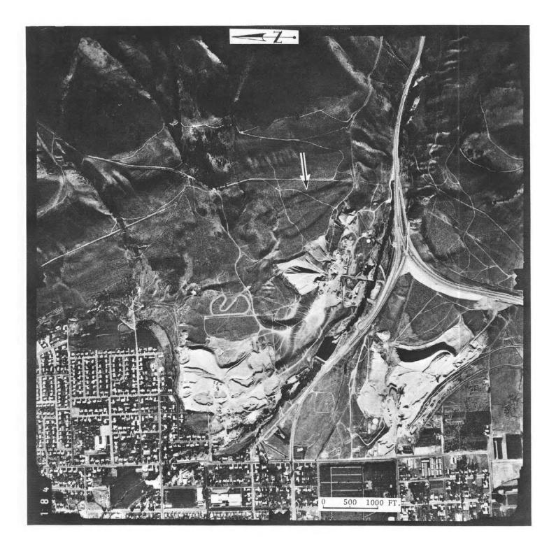
FIGURE 9. The Wasatch fault at Brigham City, Utah. This Low-Sun-Angle aerial photograph shows large-scale landsliding with faulting east of Brigham City. The area of landsliding is indicated by the arrow; landslide scarps cast linear shadows that show as dark lines on the photograph.
