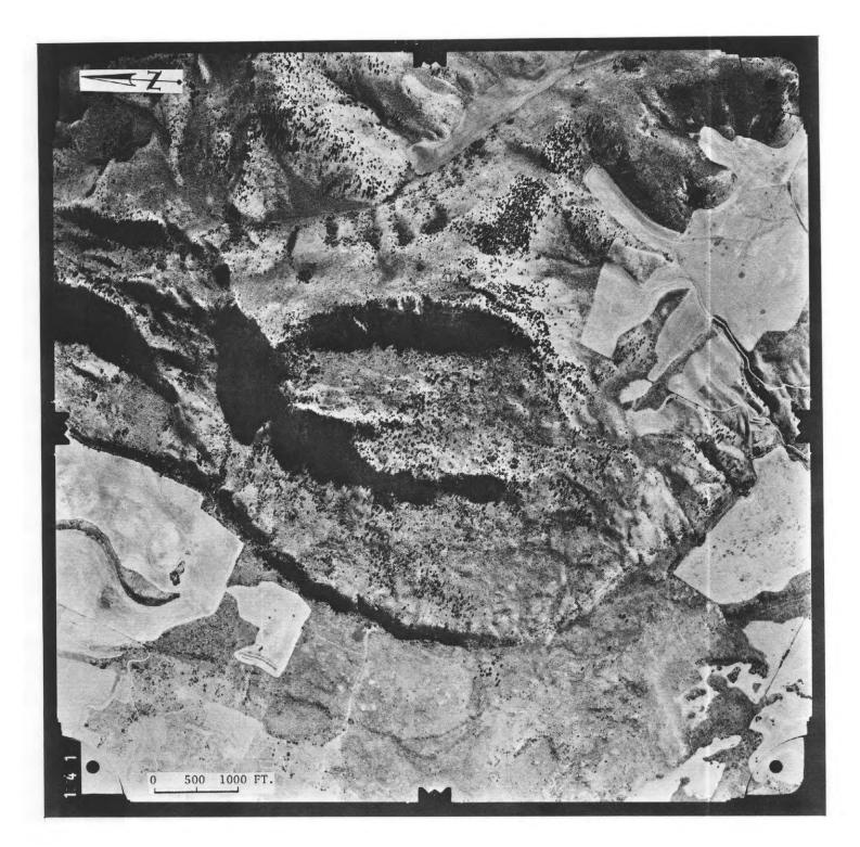
FIGURE 13. Vertical aerial photograph of the west slopes of the Junction Hills. Landsliding is evident in this area, and large boulders derived from the landslides cover the gentle slopes in this area. The elongate breaks in slope are shorelines.
