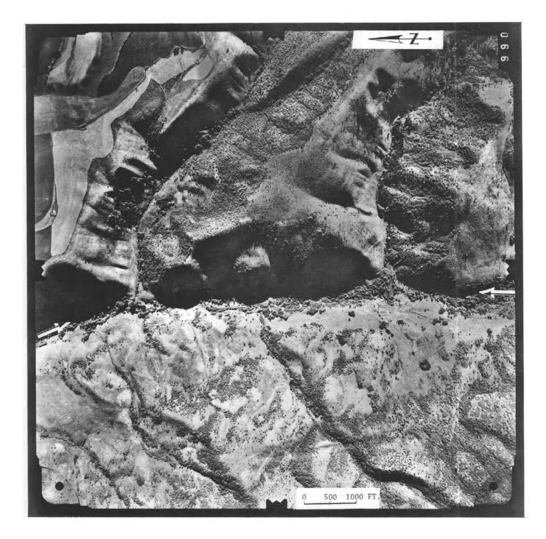
FIGURE 17. Vertical aerial photograph of the East Cache fault along Davenport Creek. The fault, indicated by arrows, is followed by the Creek, which has eroded the most recent fault scarplets.
