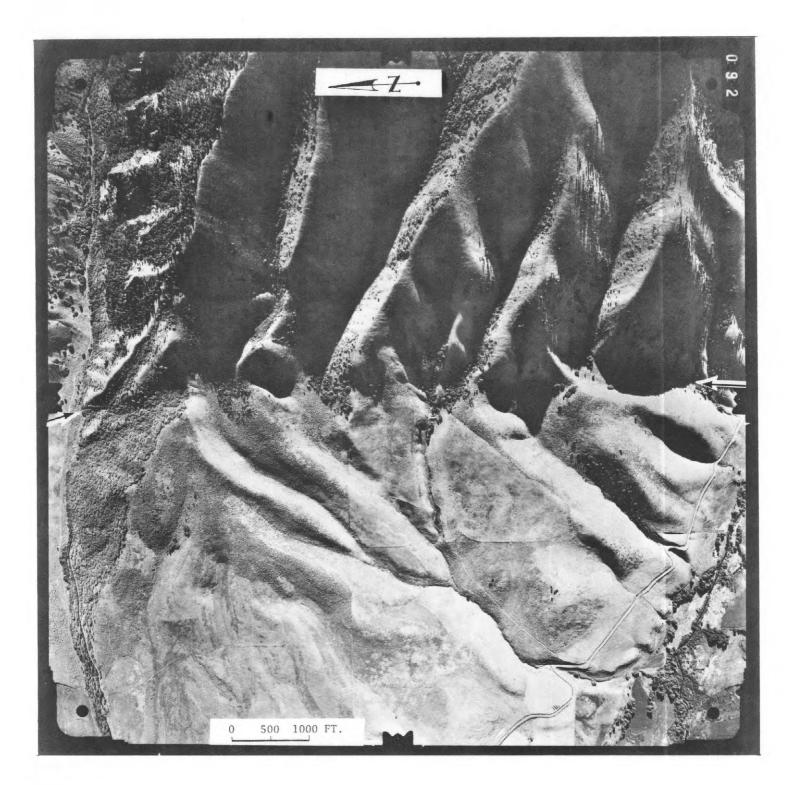
FIGURE 19. Vertical aerial photograph of the East Cache fault South of Logan, Utah. The most recently active fault trace forms the prominent west-facing slopes, indicated by arrows, but the fault does not appear to displace the young alluvium in this area.
