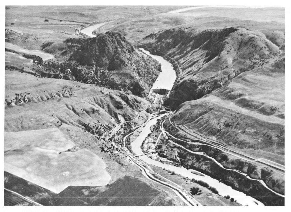
FIGURE 11. Oblique aerial photograph of Culter Dam. The view looks east. The area in the foreground was involved with large-scale landsliding that was apparently covered byLake Bonneville. Faults are apparently masked by younger landslides in this area.
