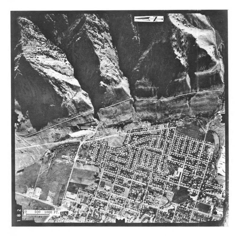
FIGURE 7. The Wasatch fault at Brigham City, Utah. The view of this vertical Low-Sun-Angle aerial photograph is the same as the right foreground of Figure 6. The most recent fault scarps, marked by a sinuous line of shadows and springs, are located between the arrows.
