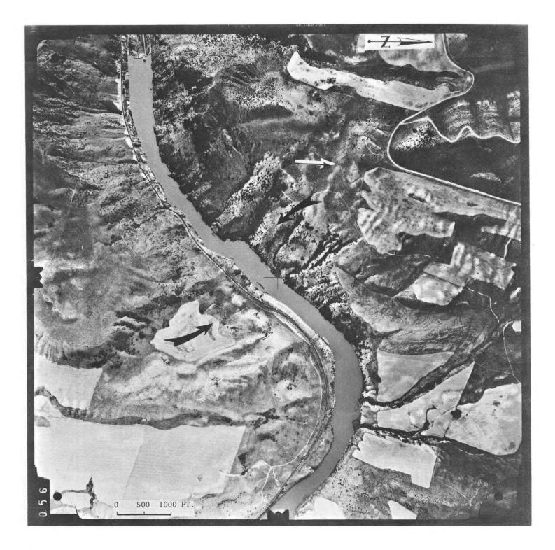
FIGURE 25. Vertical aerial photograph of the West Cache fault at Cutler Reservoir. Active traces of the fault are subdued in this area (one is indicated by the straight arrow), which is dominated by landslides, some of which are indicated by the curving arrows within the landslides.
