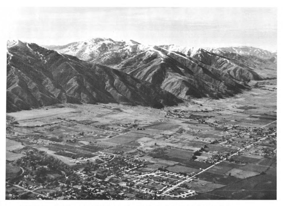
FIGURE 20. Oblique aerial photograph of the East Cache fault South of Logan, Utah. View is southeast, Providence is in the foreground. The most recently active traces of the fault are subdued, but generally at the base of the Bear River Range.
