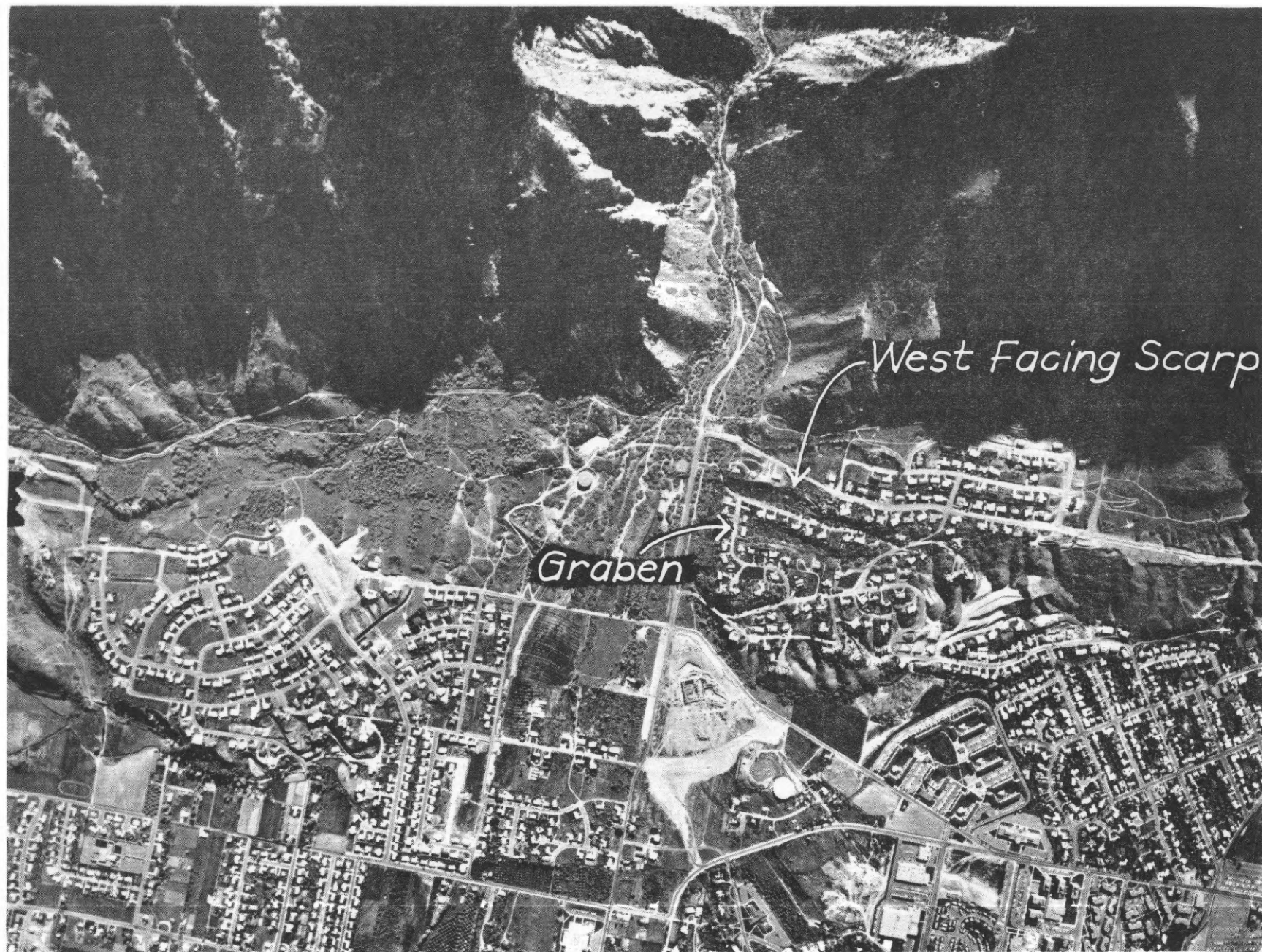
Figure 6 - Vertical aerial photograph of faulting through subdivision south of Rock Canyon. Approximate scale 1:12,000.
