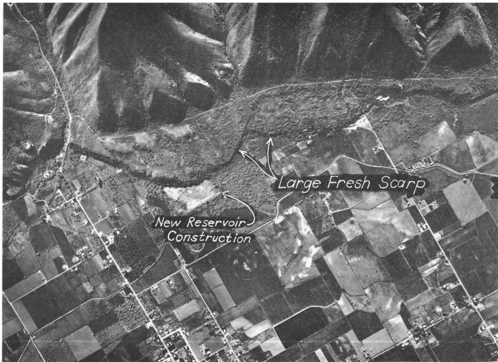
Figure 10 - Vertical aerial photograph showing faulting through new reservoir construction south of Maple Canyon. Approximate scale 1:12,000.
