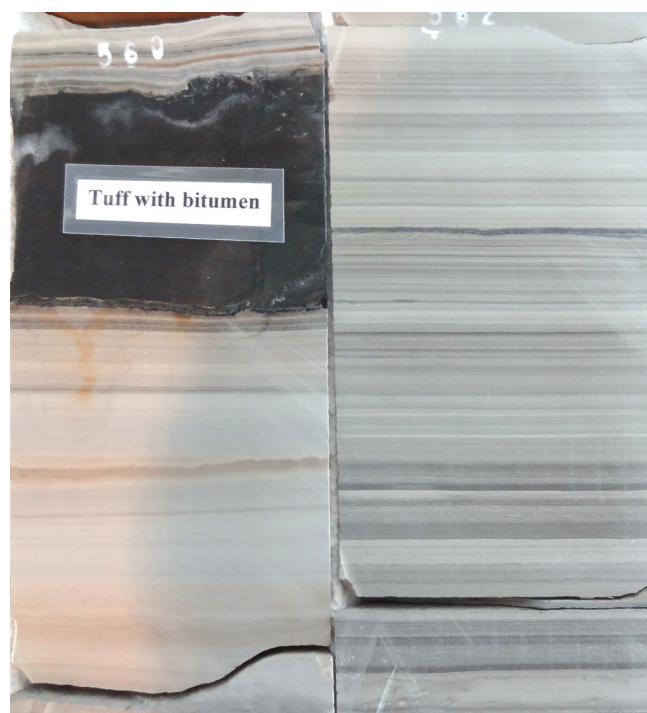
Figure 3-17: Bitumen impregnated tuff bed in the upper R-6 oil shale interval in the Skyline 16 core. The tuff bed is just 2 inches thick. The core is southeast of the WOSCO EX-1 core in 10-11S-25E; UTM E 661445, UTM N 4415109.
