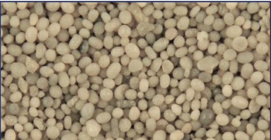
A magnified photo of oolitic sand; width of view is about one-fourth of an inch. Photo by Paul W. Ramsey.
