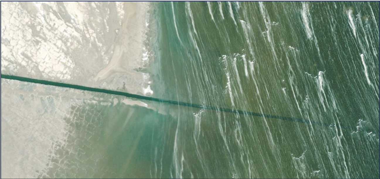
The Behrens Trench flows from a brine pond eastward, into and beneath Great Salt Lake. In this image the canal is about 60 feet wide and spans 1.3 miles. Top of photograph is oriented to the north. Photo courtesy of the U.S. Department of Agriculture, Farm Service Agency.
