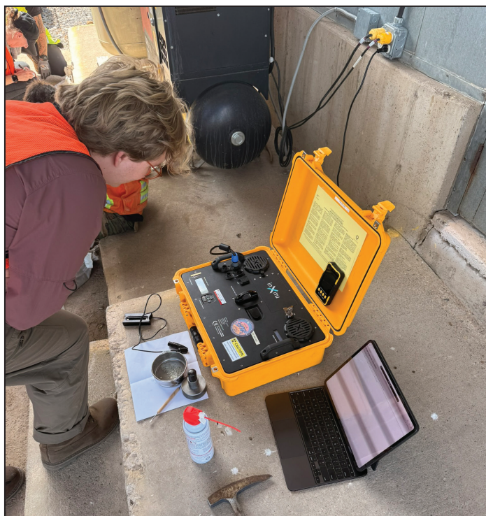
Geologist monitoring a portable dual XRD/XRF (X-ray diffraction/X-ray fluorescence) instrument, which is being used to identify mineralogy and geochemistry from downhole mine waste samples at the historic Burgin mine.
