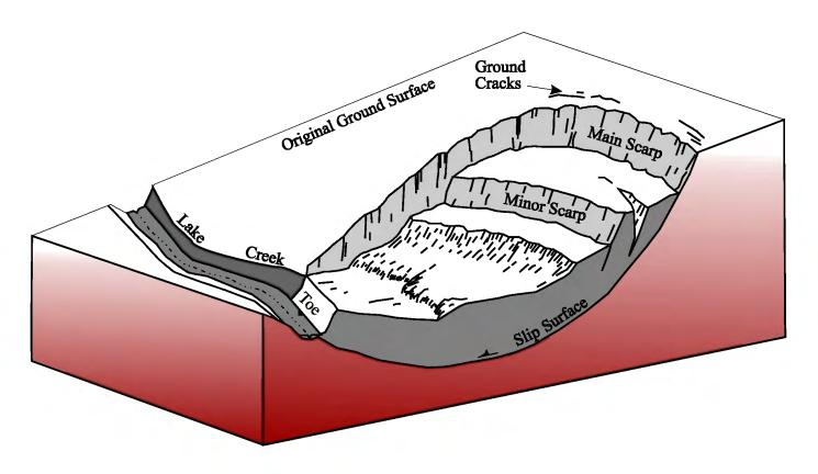
Figure 2. Conceptual diagram showing main features of landslides at Timber Lakes Estates.
