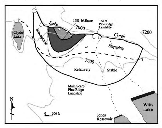
Figure 3. Map showing area susceptible to slumping. Results of our analyses suggest northern part of landslide is susceptible to slumping at high groundwater levels even if soil strengths approach their highest values. Boundary is based on using average strength value. Shaded area surrounding boundary is zone of uncertainty regarding actual location of boundary. Dotted line shows recommended setback from main scarp of 1985-86 slump. Elevations in feet above mean sea level.
