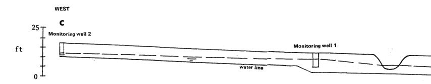
Cross sections showing water-table configuration on 9/24/84.
