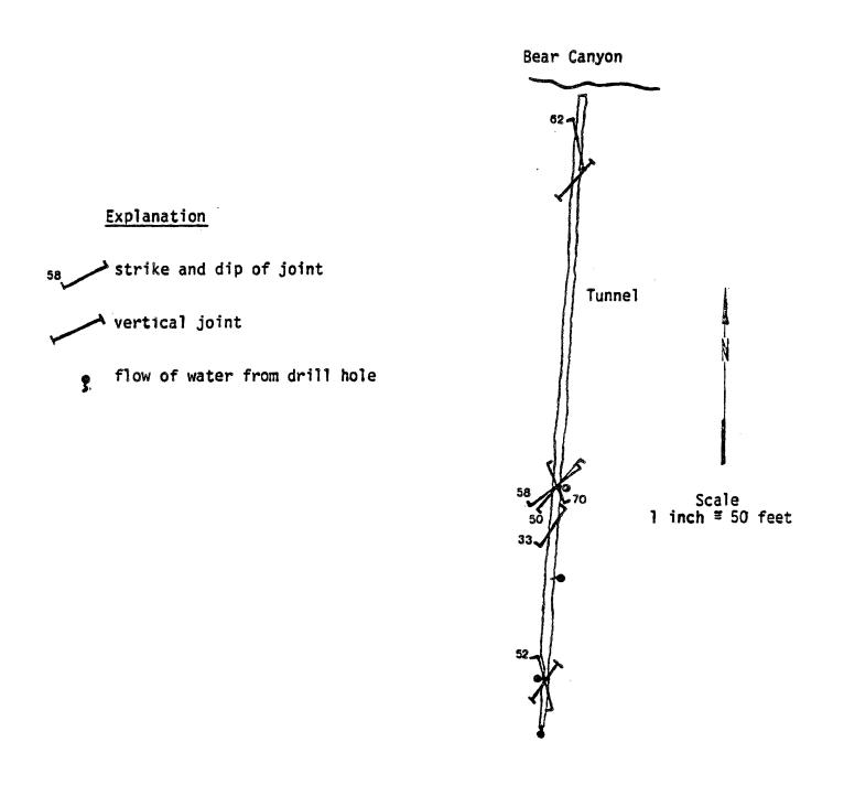
Approximate locations of joint measurements and flow of water from drill holes, Riverton Spring tunnel in Bear Canyon
