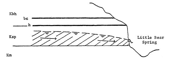
B. Confined (artesian) conditions in the Star Point Sandstone, Hiawatha seam acting as an aquiclude or confining layer
