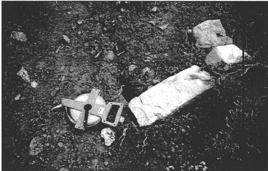
Attachment 7. Separation across a ground crack downslope and west of the graben. Separation across the crack increased from 3-1/8 inches on May 28 to 3-1/4 inches on June 4.
