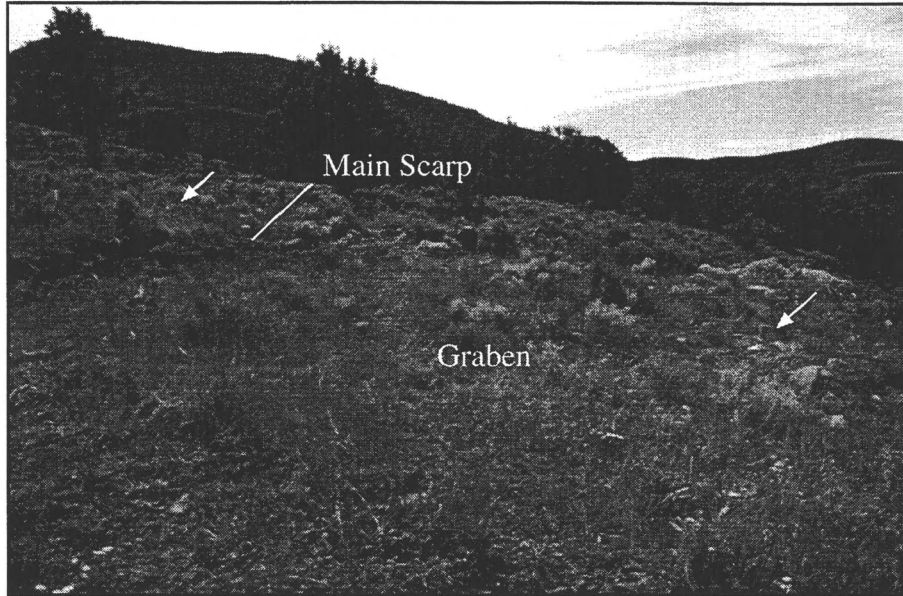
Attachment 8. Stakes installed by Utah Geological Survey to monitor movement of landslide. Upslope stakes (arrows) span main scarp of the graben. Although separation across the main scarp locally increased by as much as 4-1/2 inches over the period between May 28 and June 4, subsequent surveying by Summit County has indicated no discernable movement of the slide despite periodic heavy rain. View is to the southwest.
