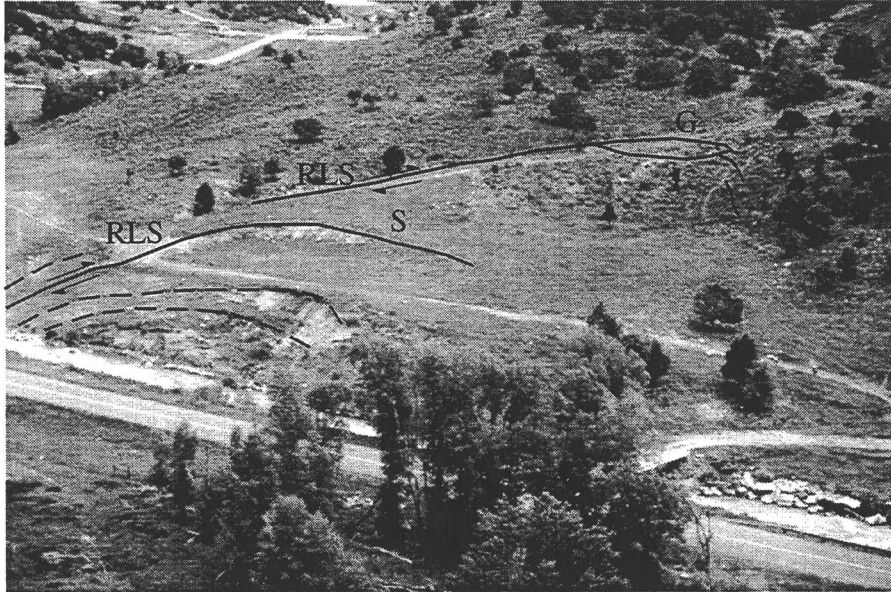
Attachment 2. Oblique view of landslide along Chalk Creek. Active landslide features (solid lines) include the scarps bounding the graben (G), right-lateral scarps (RLS), and main scarp of the uppermost slump (S). The extent of recent movement of the lower slumps and lower part of right-lateral scarp (dashed lines) is uncertain. Traces of all features are approximate and representation of ground cracks near graben is schematic. View is to the east.
