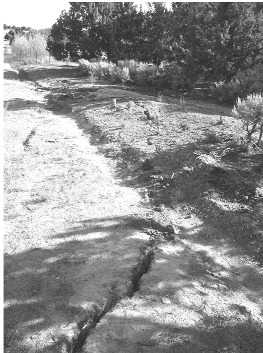
Figure 4. Crack on east side of the house, near or above the septic-tank drain field. View to the north.
