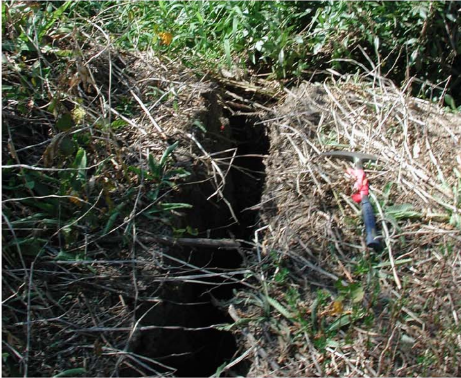
Figure 7. Ground crack in the south bank of South Fork Kays Creek on August 27, 2001. Crack width is 6 inches.
