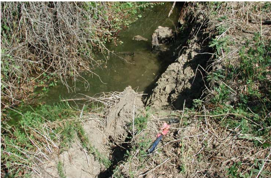
Figure 8. Toppling of the south bank into South Fork Kays Creek on August 27, 2001. Landslide movement is from right to left, view looking upstream to the east, rock hammer for scale.
